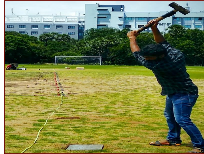
Surface wave testing
