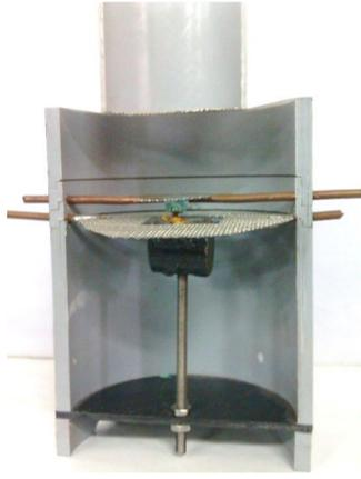
Developing short-term test methods for reliably determining the chloride threshold and corrosion rate
