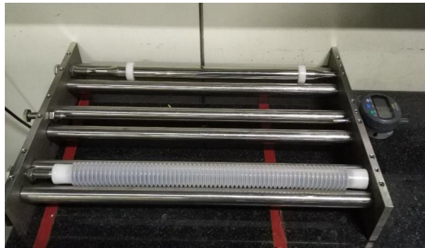
Corrugated tube for early-age autogenous shrinkage
