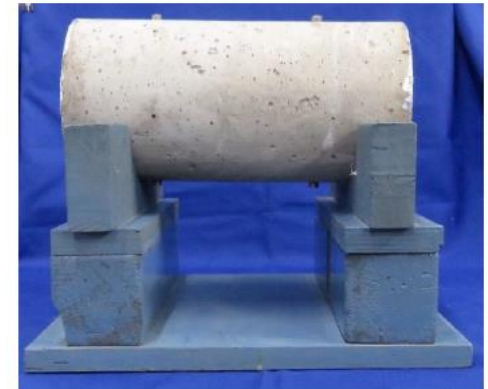
Concrete cylindrical specimen with studs in place
