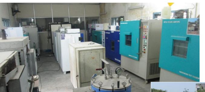
High-temperature, carbonation, humidity chambers
