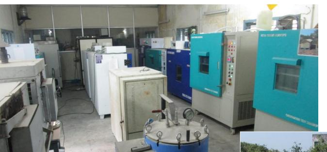
High-temperature, carbonation, humidity chambers
