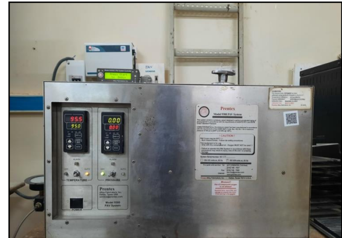
Prentex, USA: Pressure Aging Vessel
