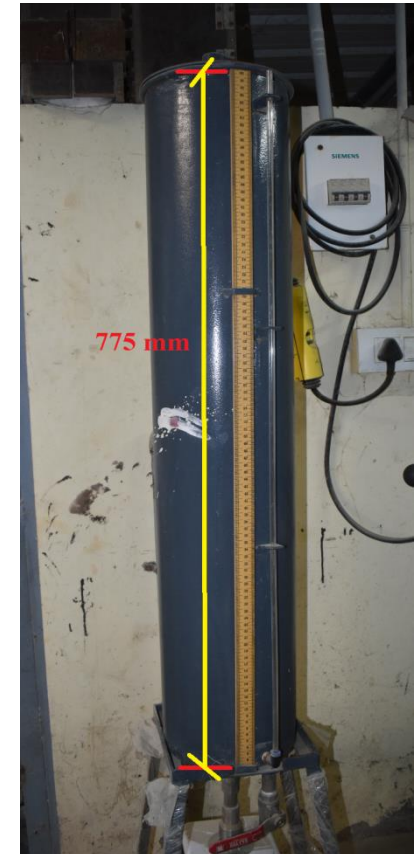
EIE instruments, India: Constant Head Water Sprayer
