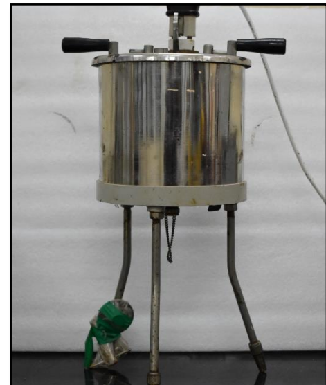
HEICO, India: Saybolt Furol viscometer
