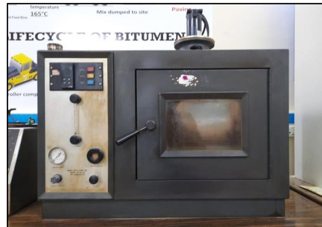
Cox & Sons, USA: Rolling thin film oven
