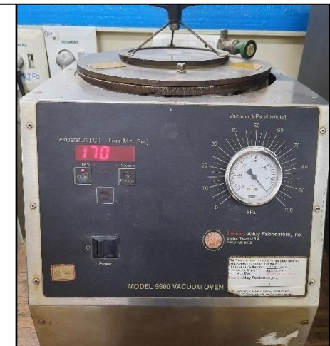
Prentex, USA: Degassing oven
