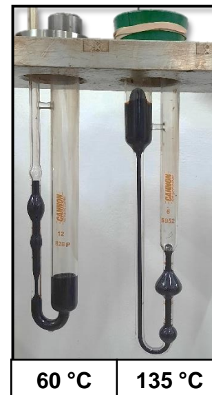
Cannon Instrument company, USA: Viscometer
