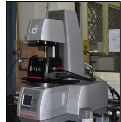
Courtesy: Anton Paar, Germany. DSR MCR 702
