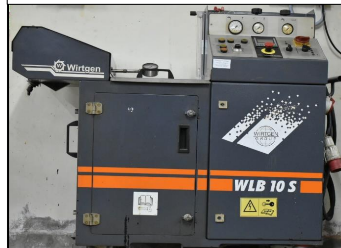
Wirtgen, German: Foaming equipment: WLB 10 S
