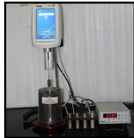
Brookfield, USA: Rotational Viscometer
