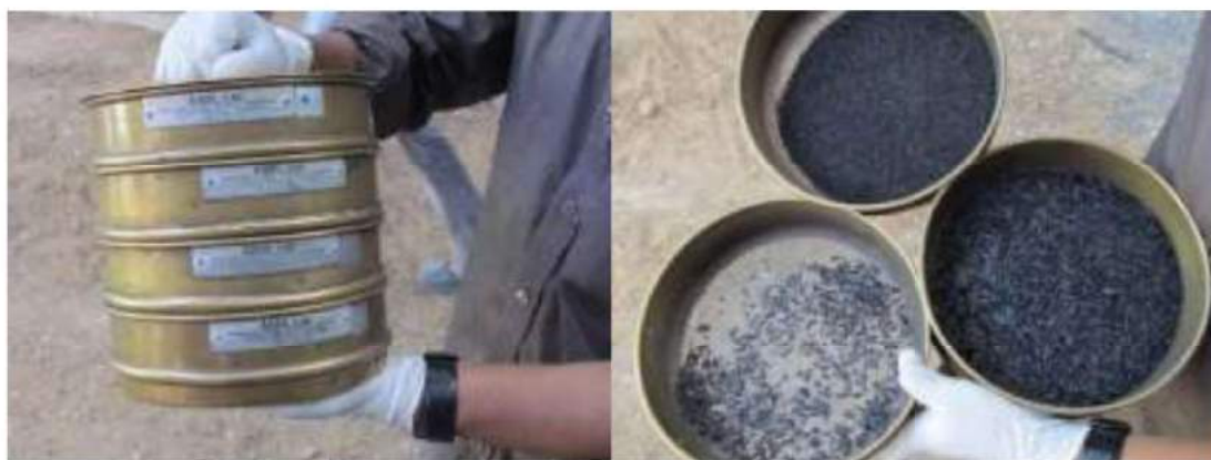
Figure 4.2: Separation of different particles from raw SCBA by sieving
