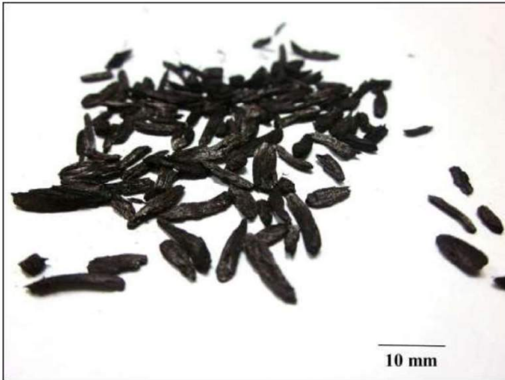
Figure 4.3: Coarse fibrous unburnt particles (CFU) present in the bagasse ash sample
