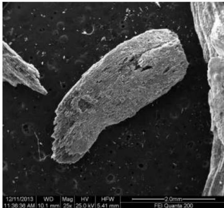
Figure 4.31: Microstructure of coarse fibrous particles
