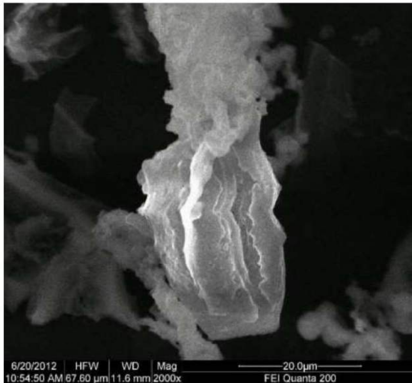
Figure 4.27: Microstructure of fine burnt particles
