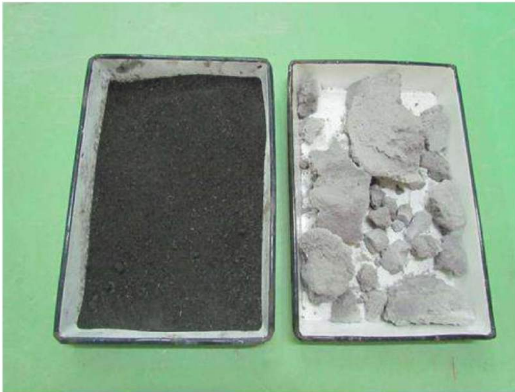
Figure 5.15: Raw bagasse ash (left) and white particles at 900 °C (right)
