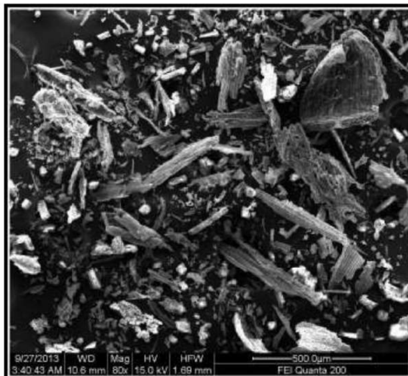
Figure 5.10: Presence of fibrous carbon particles in 700 °C burnt sample
