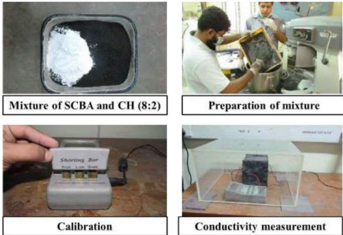
Figure 4.13: Preparation of hydrated lime-pozzolan mixture and electrical conductivity measurement
