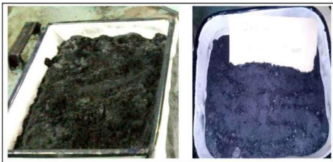
Figure 5.4: Appearance of bagasse ash burnt at 30 min (left) and 75 min (right) respectively
