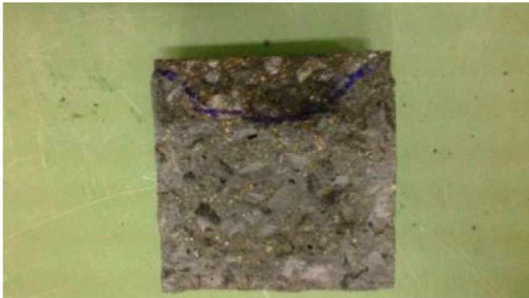
Figure 7.17: Depth of water penetration
