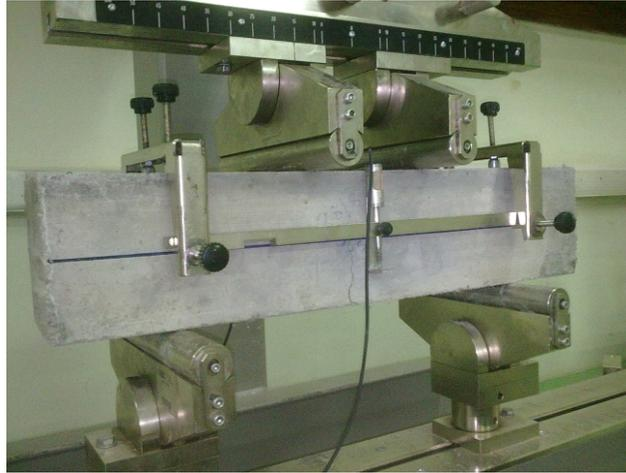
Figure 3.8: Third point loading test configuration
