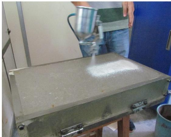
Figure 7.1 Application of curing compound
