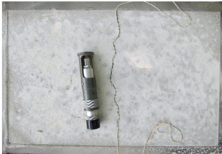
Figure 3.5: Measurement of crack width and length
