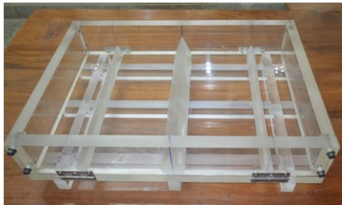
Figure 3.3: Plastic shrinkage mould
