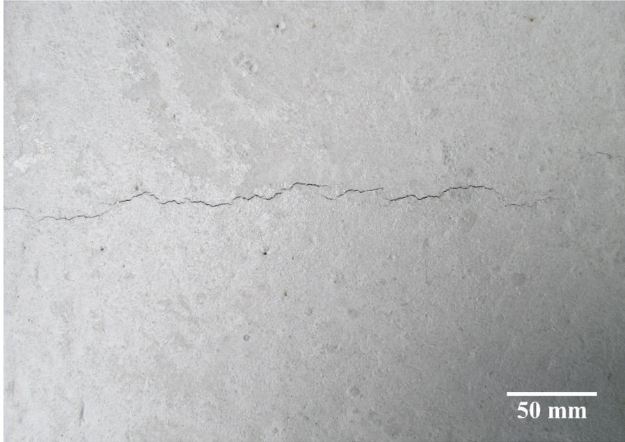
Figure 4.10: Plastic shrinkage cracking in FA30
