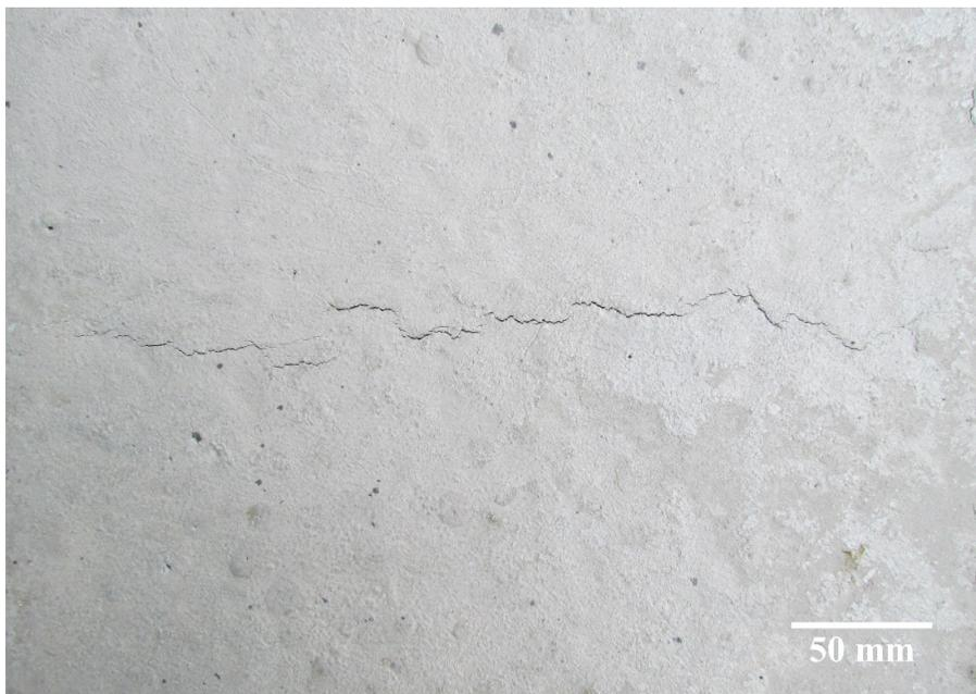
Figure 4.9: Plastic shrinkage cracking in FA15
