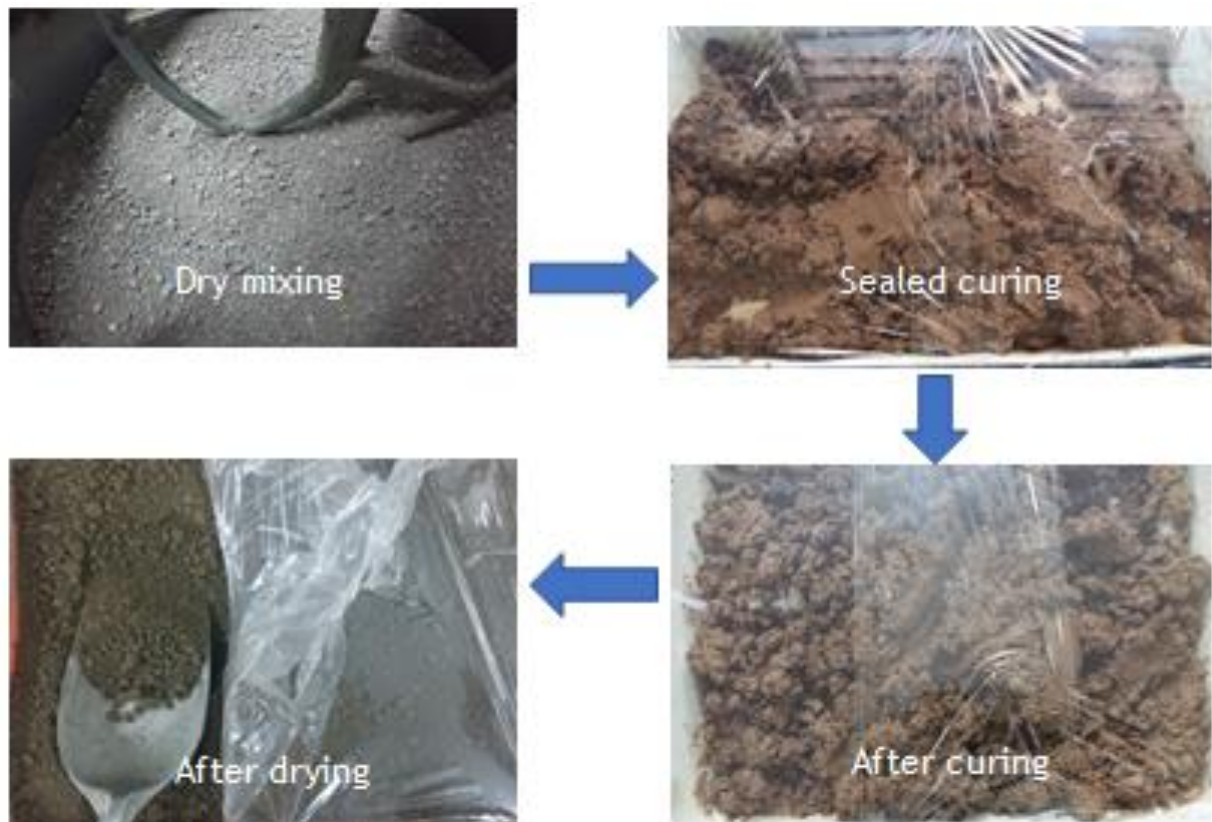
Figure 5.2 Soil stabilization process
