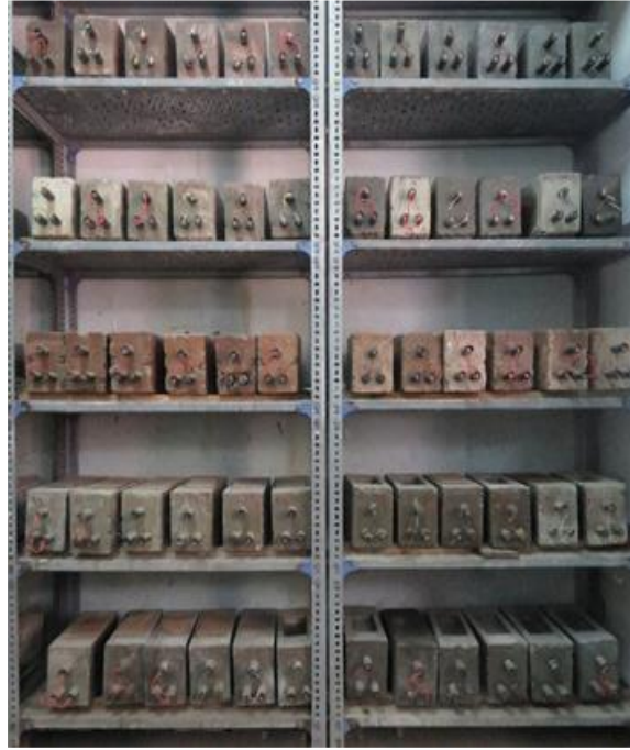
Figure 4.1 ASTM G109 specimens being exposed
