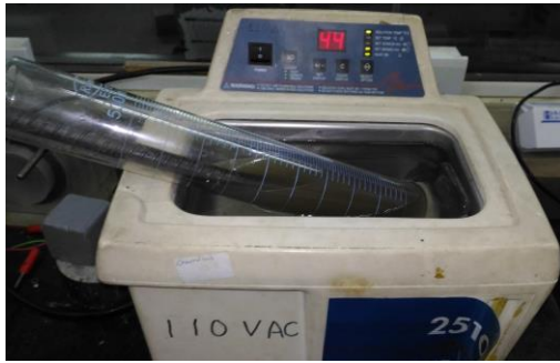
(a) Cleaning in ultrasonic cleaner
