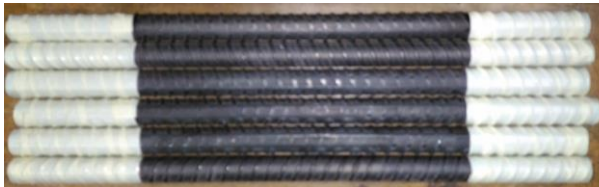
(c) Ends wrapped with electroplaters tape
