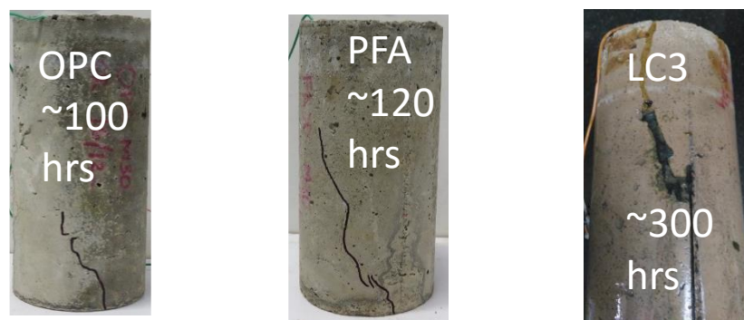
Figure A.5 Specimens showing crack and corrosion products in M35 concrete (Case III)
