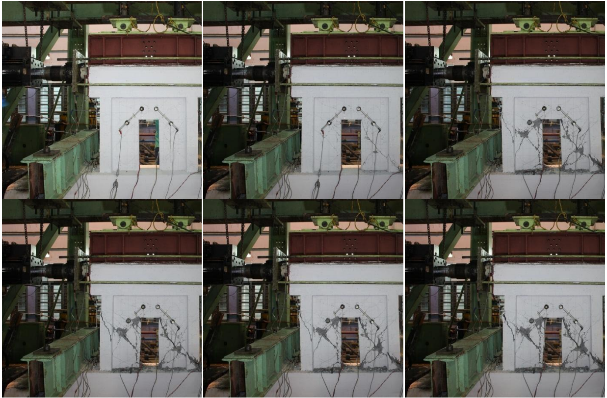
Fig. 5.20 Failure Stages for SW-1.0-CD-00
