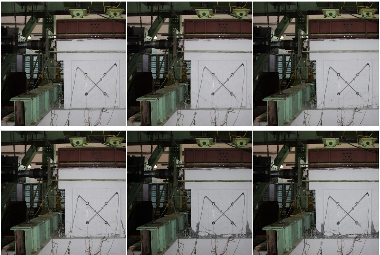
Fig. 5.17 Failure Stages for SW-1.0-00-00
