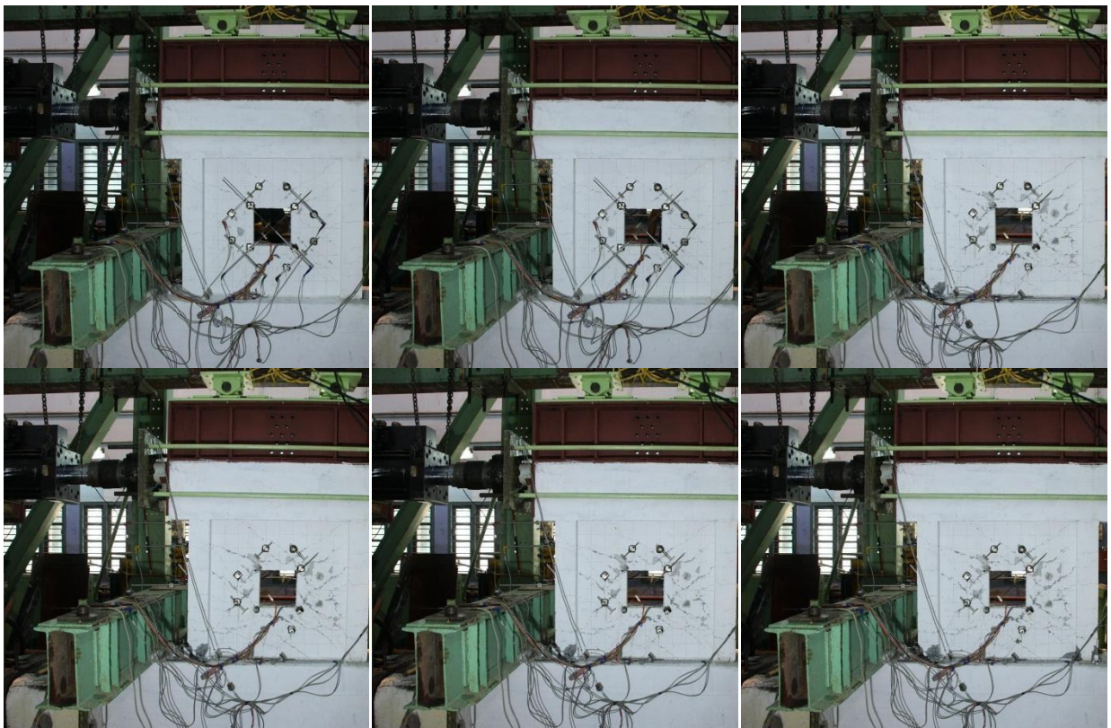
Fig. 5.19 Failure Stages for SW-1.0-CW-FRC
