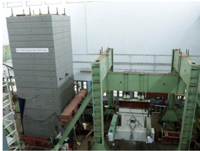
Fig. 4.18 Test Setup for shear wall
