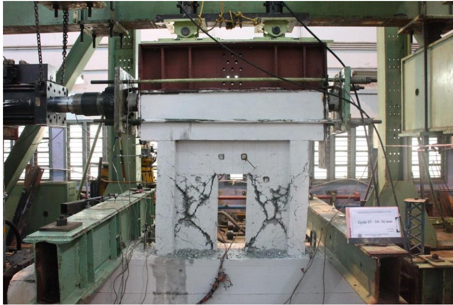
b. At the Failure load
