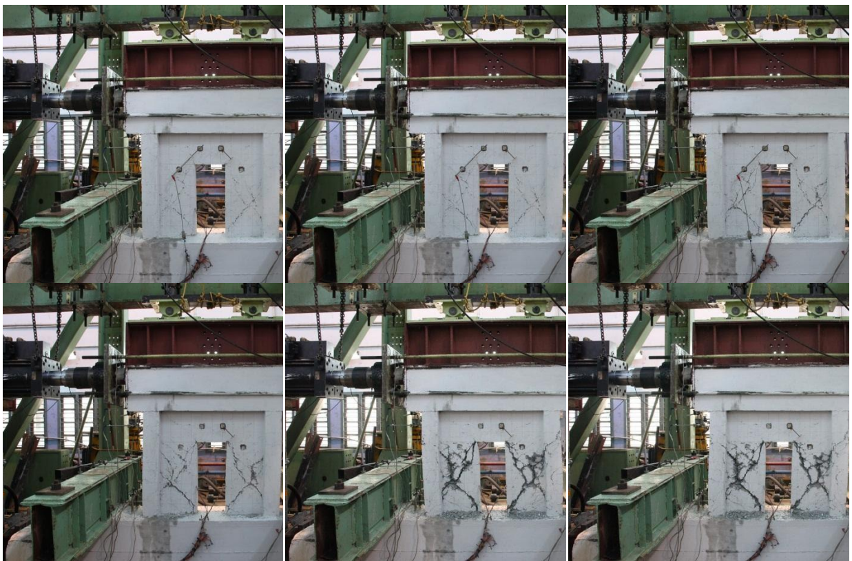
Fig. 5.21 Failure Stages for SW-1.0-CD-FRC
