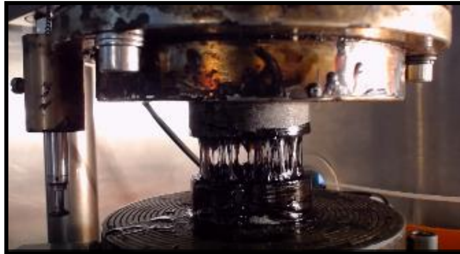
IPC global, Australia: Pull-off testing jig
