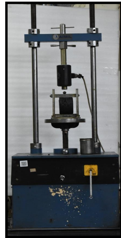
AIMIL, India: Indirect tensile test apparatus
