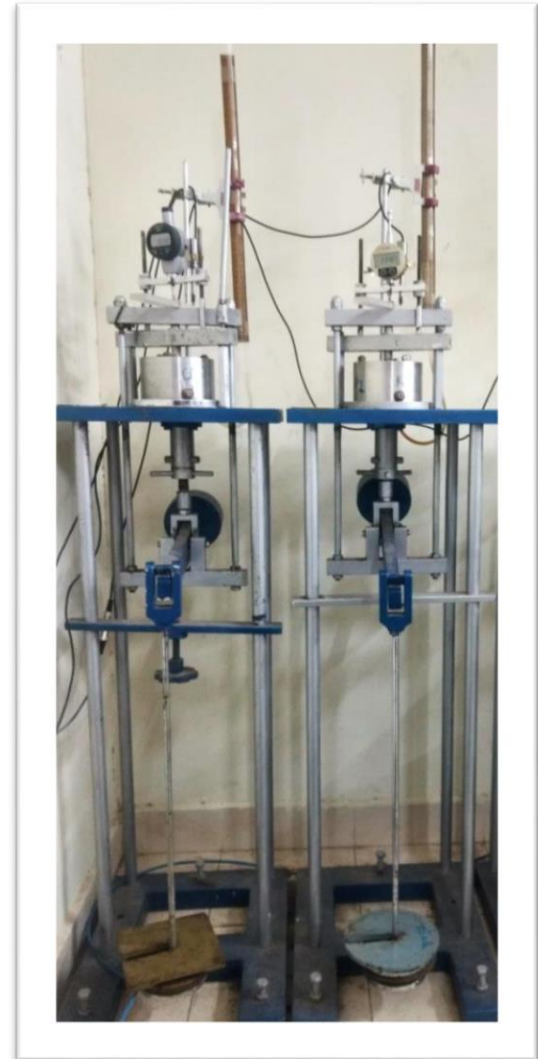
One-Dimensional Consolidation Test
