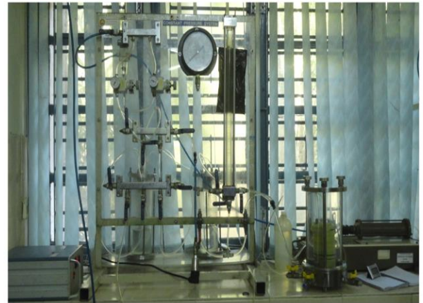
Flexible Wall Permeability Test
