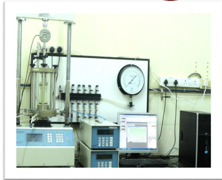
VJ Tech Triaxial Testing Equipment
