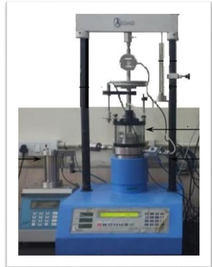
CRS Consolidation Test
