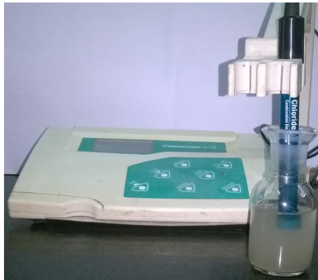
Figure 8.1 Steps for determining chloride threshold of steel-mortar interface
