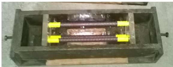
(e) CPC coated rebar cage placed in mould
