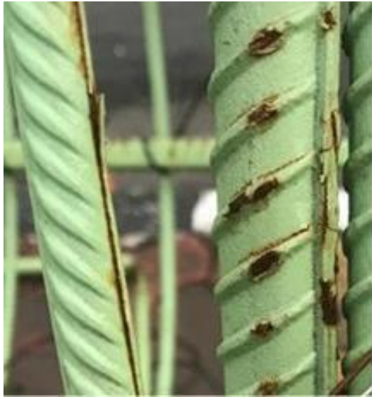
(a) Scratch damage and disbondment of the coating due to poor handling of rebars at sites
