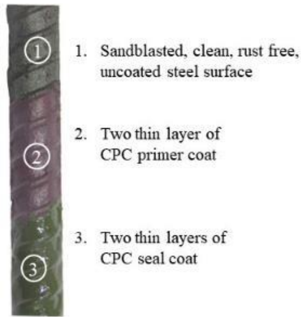
Figure 2.16 Typical steps for CPC coating
