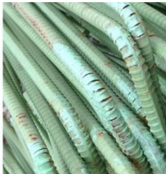
(b) Cracked FBE coating at the cracked locations
