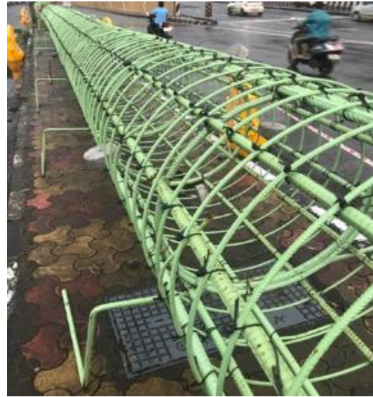
(b) Exposure of coated steel to sunlight during storage or delayed construction
