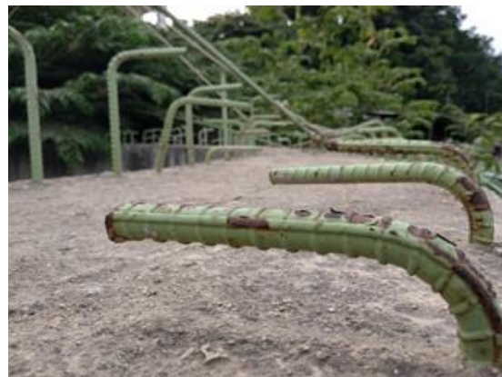
(b) Close-up showing damaged FBE coating steel rebars being used
