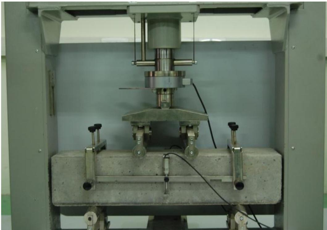
Figure 3.1 Flexural toughness test setup
