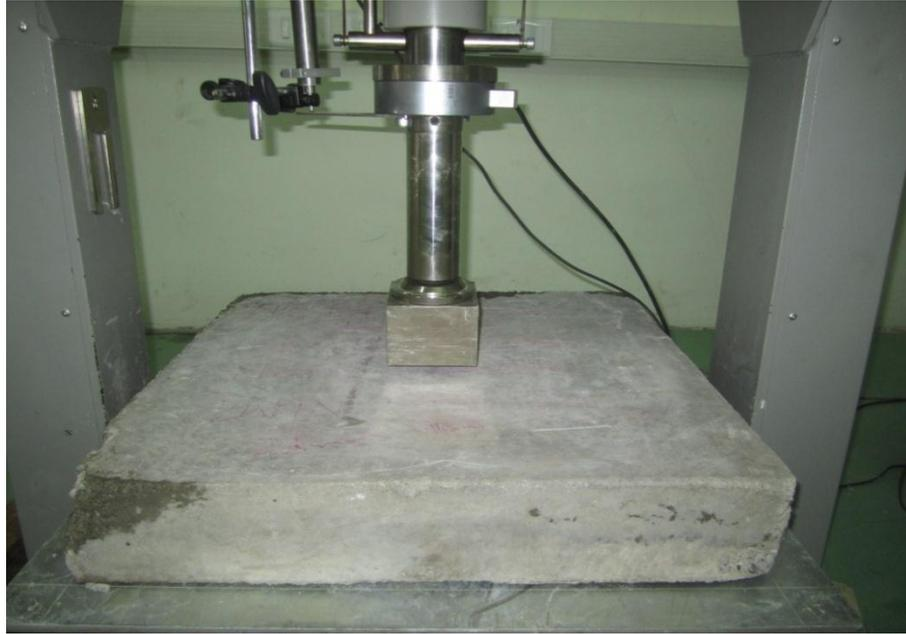
Figure 2.1 Square panel testing as per EFNARC-EVS-EN 14488-5
