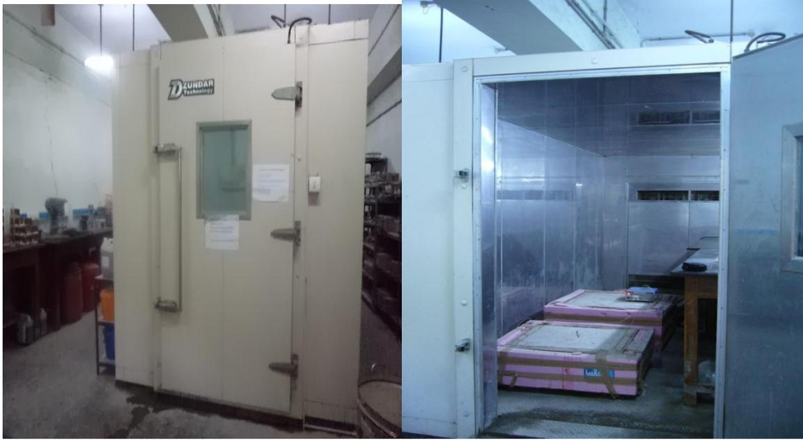
Figure D.2 Slabs placed inside the walk-in environmental chamber
