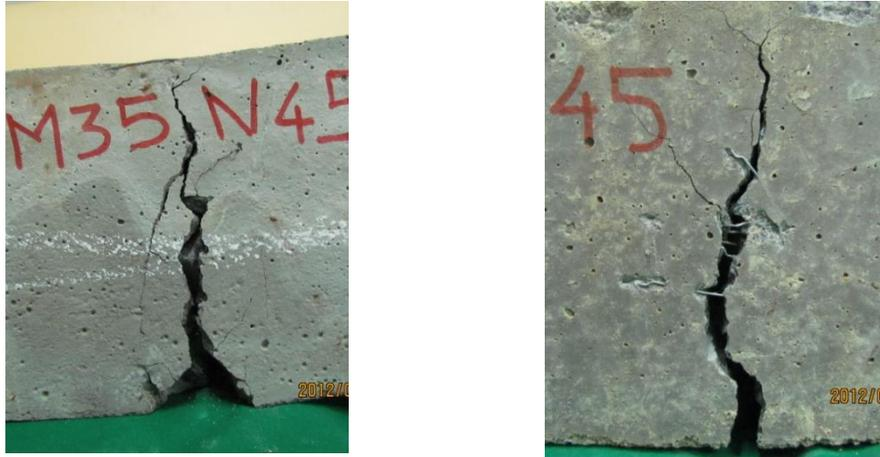
Figure 4.2 Crack pattern after the end of the beam test: (a) larger damaged area in concrete with SFC fibres and (b) single major crack in concrete with SFB fibres
