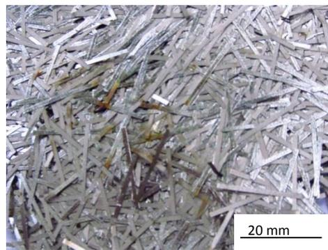
Figure 5.3 Fibres after 4 weeks of immersion in 3.5 % NaCl solution.
