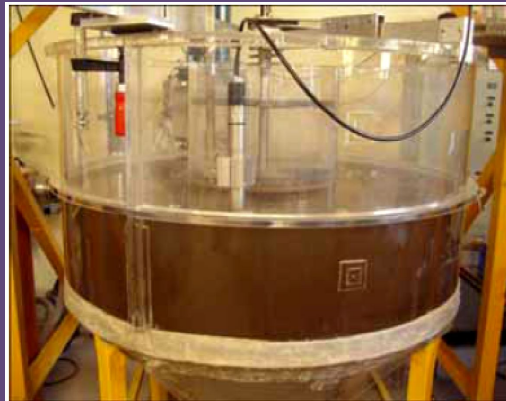
Annular flume (Cohesive sediment studies)
