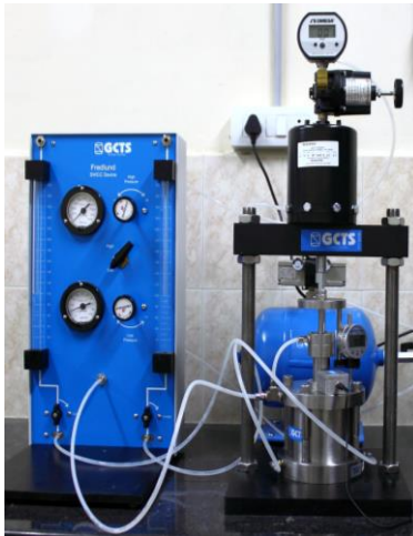
GCTS SWC-150 Cell with pressure panel and pneumatic loading frame
