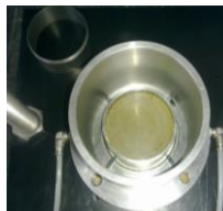
GCTS SWC-150 Cell with pressure panel and pneumatic loading frame
