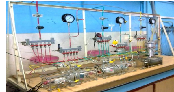
Pressure Control Panel for Gas Diffusion and Permeability Determination
