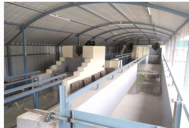
New hydraulics laboratory with experimental flumes
