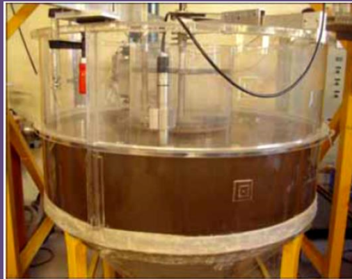
Annular flume (Cohesive sediment studies)
