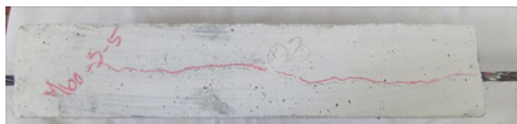
Fig. 4 Longitudinal cracks along the 7-wire strand in M55 grade in concrete
