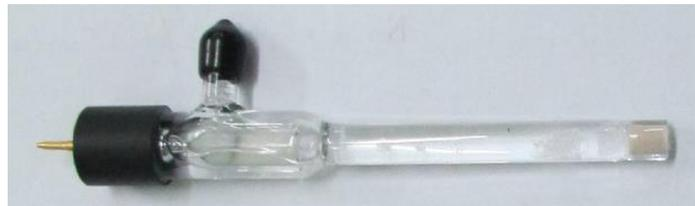
**Figure 4.11 Saturated calomel reference electrode**
