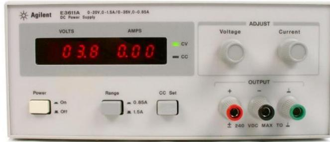
**Figure 4.3 DC potential source used for this study (Agilent E3611A)**
