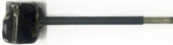
**Figure 4.13 A typical working electrode used for mACT testing**
