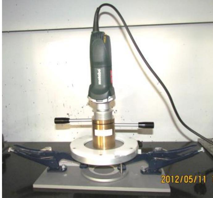
**Figure 4.20 Concrete profile grinder (Germann Inc. Model No. PF-1100)**
