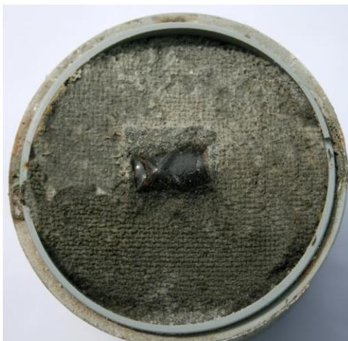
**Figure A.4 Bottom portion of the mACT specimen showing the corroded steel piece**
