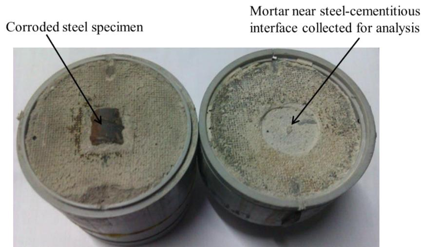
**Figure 4.19 Specimen autopsied across the steel mortar interface**
