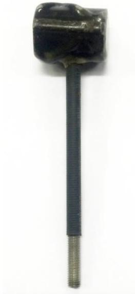
**Figure A.3 A typical working electrode used for ACT testing**
