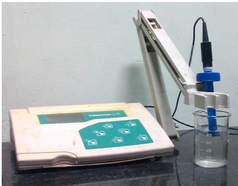
**Figure 4.5 Chloride ion specific electrode connected to conductivity meter**
