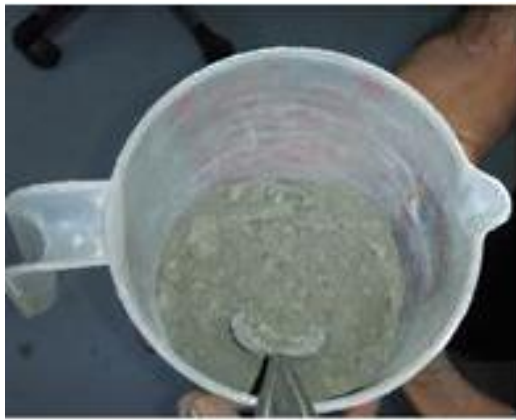
a) Binders in the container with uniform mixing
