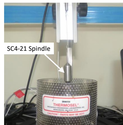
b) Co-axial cylinder and spindle attachment
