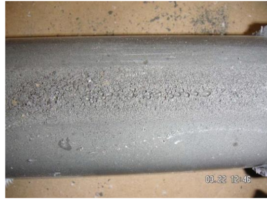
b) Porous surface texture in a commercially available PPG
