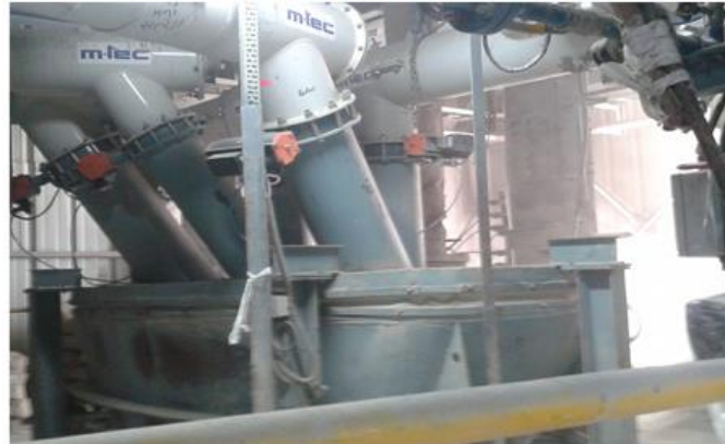
b) Blending of ingredients of PBG
