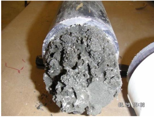
a) Porous softgrout on a hardened commercially available PPG
