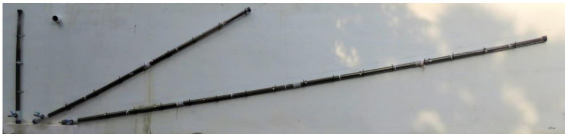
b) Prototype tendon-duct system after grouting
