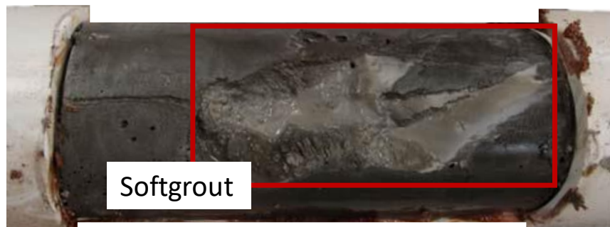
b) A scarpable layer of highly permeable softgrout (Hamilton et al. 2014)
