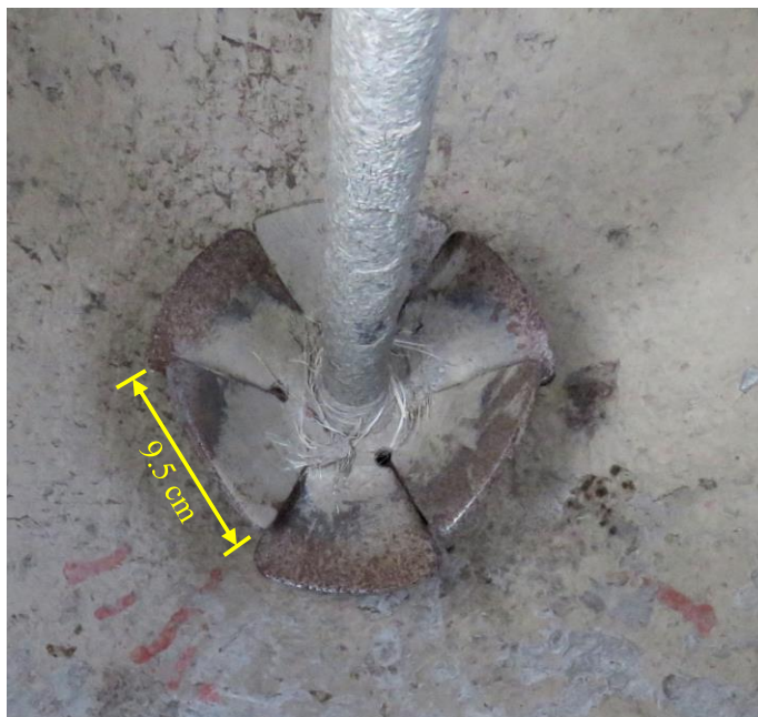
b) Mixer blade configuration
