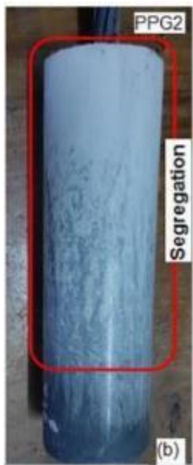
b) A scarpable layer of highly permeable softgrout (Hamilton et al. 2014)
