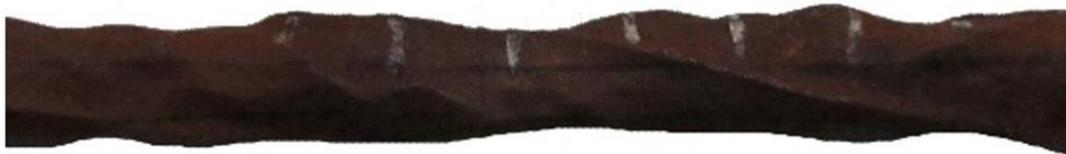
Figure 2.2 Uneven corrosion topography along the length of the rebar
