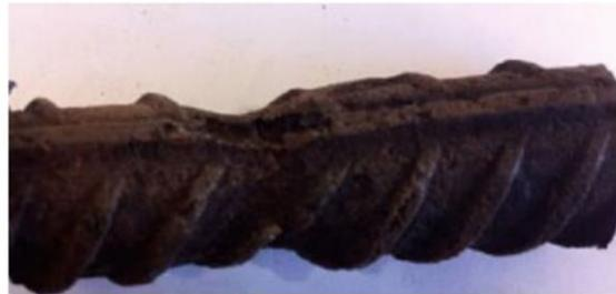
Figure 2.1 Localized (pitting) corrosion topography of the rebar (Source: Francois et al. 2012)
