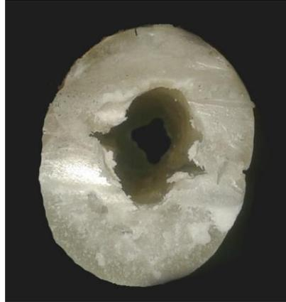
Figure 4.1 Cut surface of a wax imprint of corroded specimen revealing imperfections in the imprint
