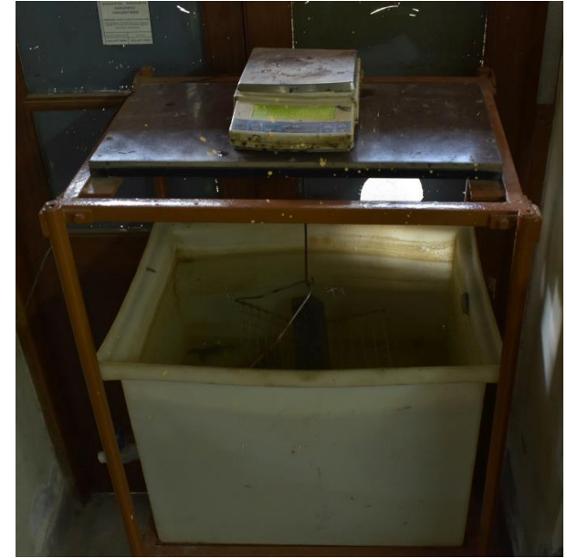
InstroTek, USA. Water tank with hanging basket and weighing balance
