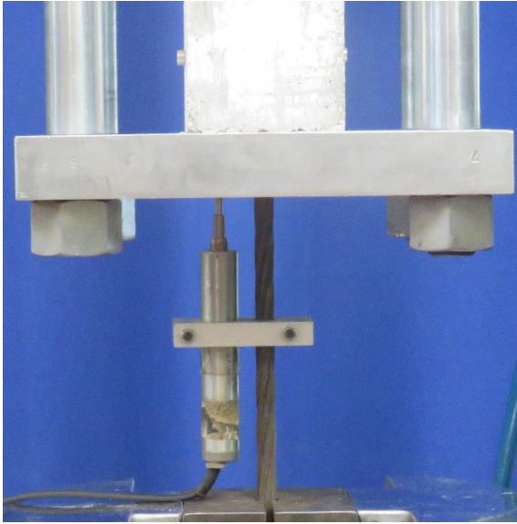
(a) In short specimens, strands get pulled-out and strands do not rupture
