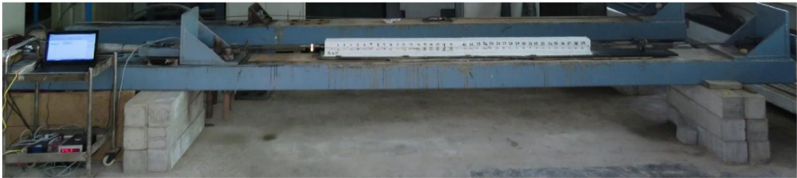
(c) Photograph of prestressing bed
