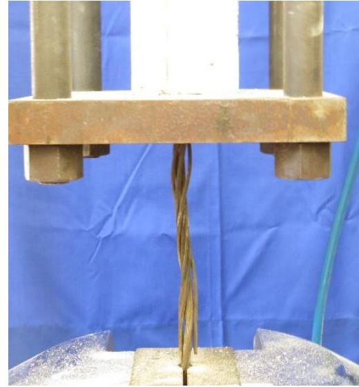
(b) In long specimens, strands get pulled-out and eventually gets ruptured
