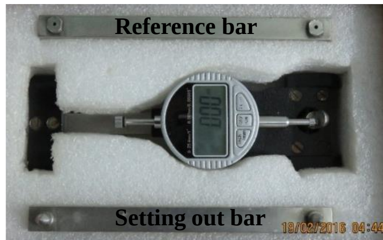
Figure 4.9 The photograph of the DEMEC gauge used to take measurements
