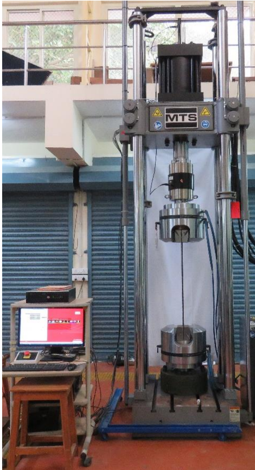
Figure 4.1 Uniaxial tensile test setup for prestressing strands
