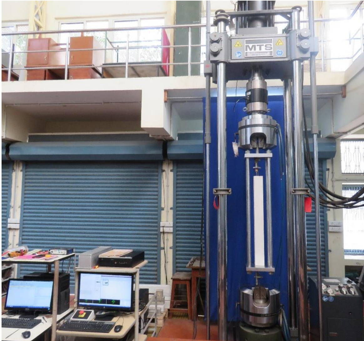
Figure 4.15 The photograph of the experimental set-up used for the pull-out test
