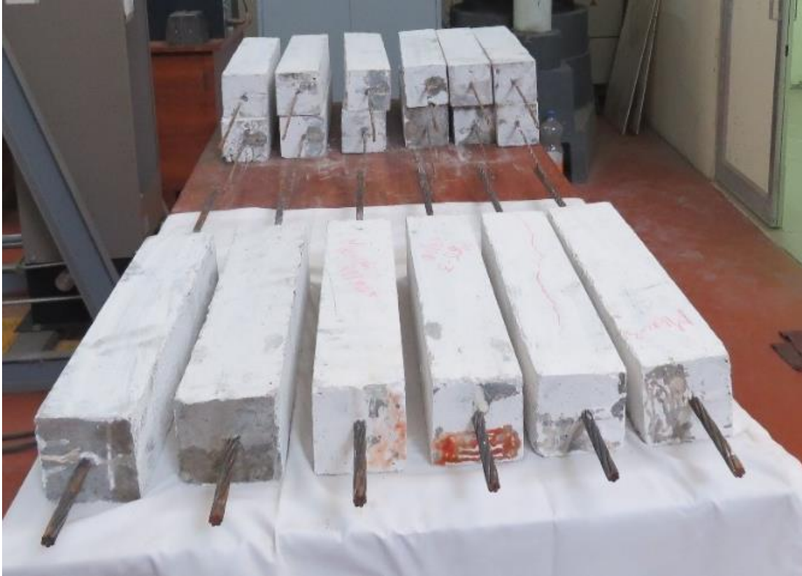
Figure 4.13 The photograph of the pull-out specimens
