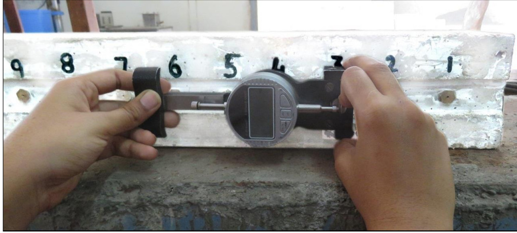
Figure 4.10 Length change being measured using the DEMEC gauge
