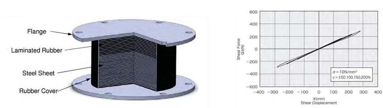
Figure 2.1 Typical elastomeric bearing system with force-displacement relationship (Li et al. 2013)
