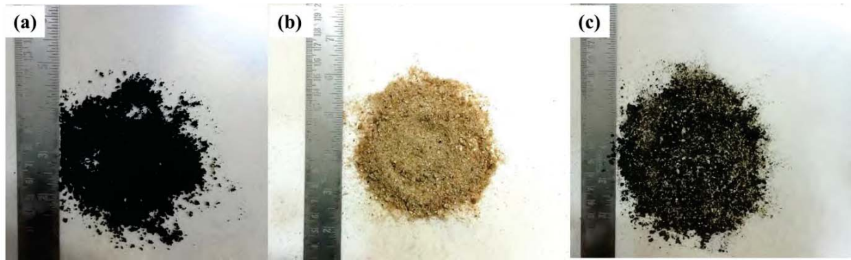
Figure 3.2 Samples of (a) Sand (b) Granulated rubber (c) SRM
