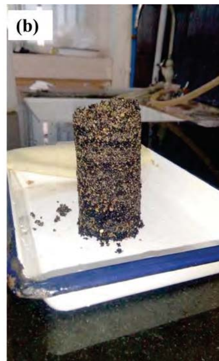
Figure 3.13 (a) Prepared SRM sample (b) No evidence of segregation
