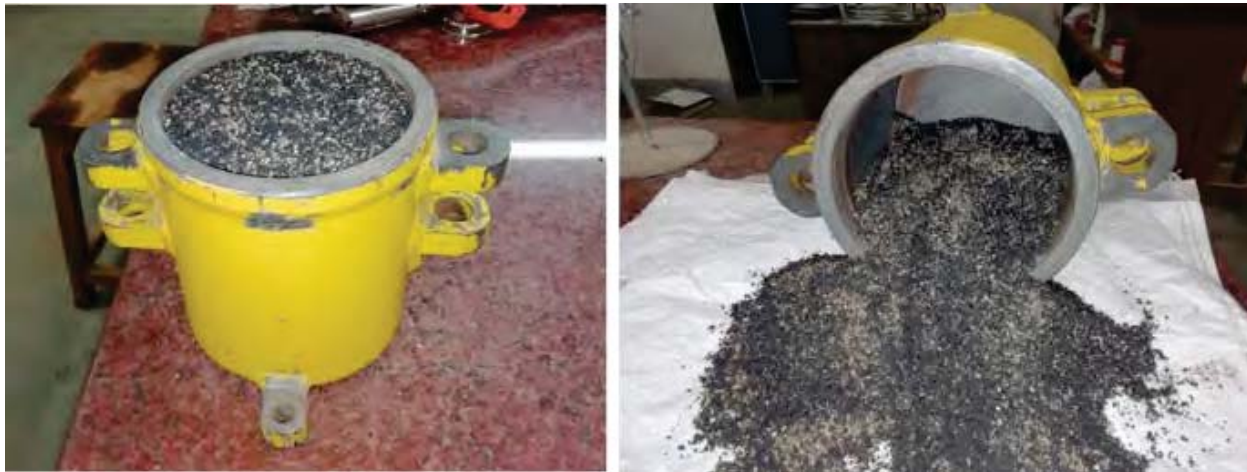
Figure 3.6 Segregation checks before and after subjected to vibration
