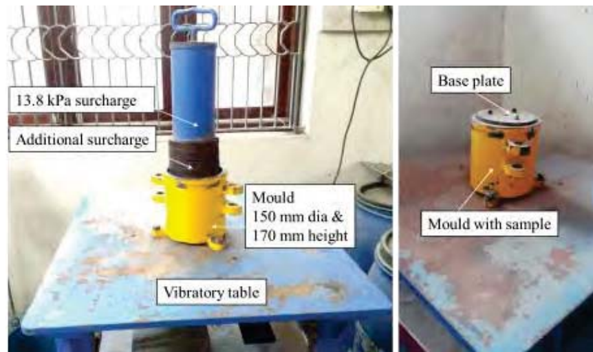
Figure 3.3 Vibratory table test setup with surcharge
