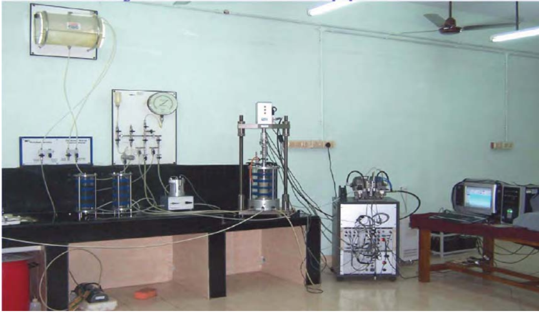
Figure 3.19 Cyclic triaxial test setup
