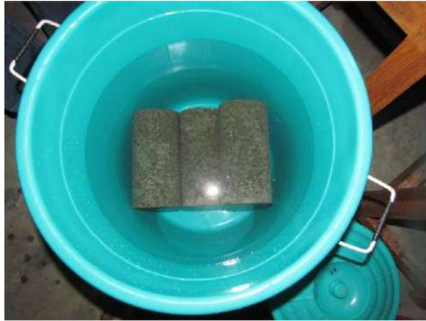
Figure 6.9 Porous concrete specimens were cured in tap water for a period of 7 days before testing
