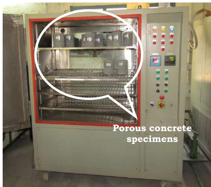
Figure 7.4 Carbonation test chamber that was used in this study
