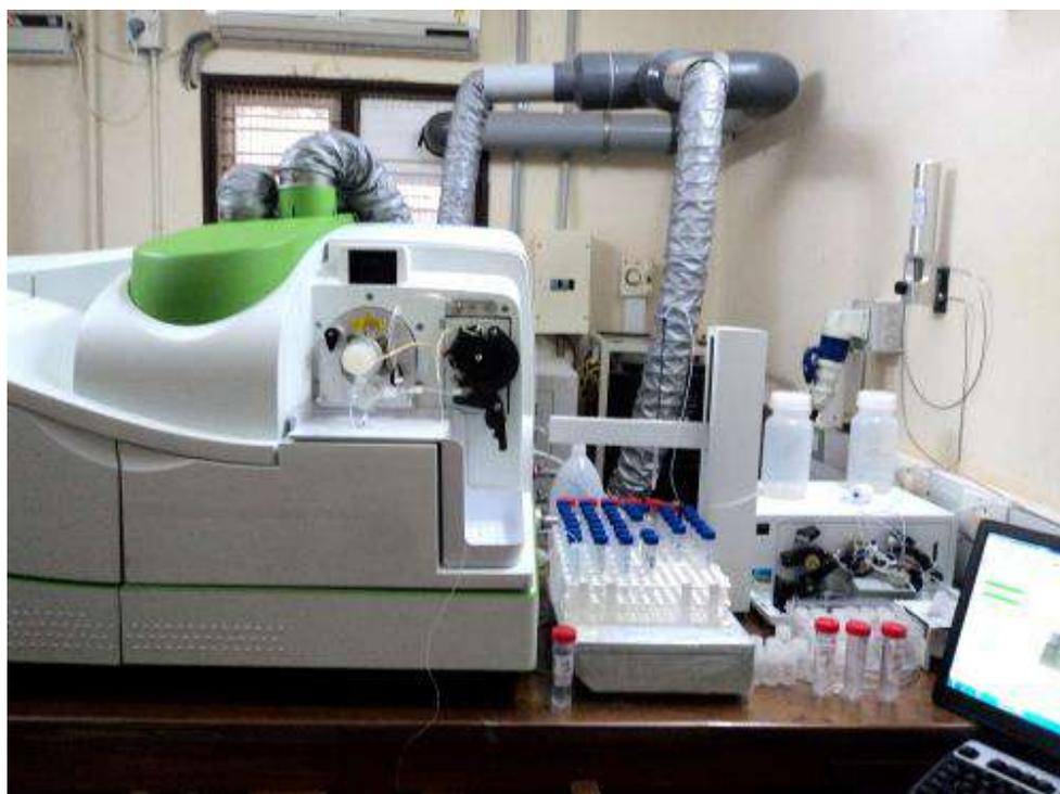
Figure 3.12 Photograph of ICP-MS (NexION 300X - Perkin Elmer. Plasma source: Argon, 18 L / min flow rate) that was used in this study
