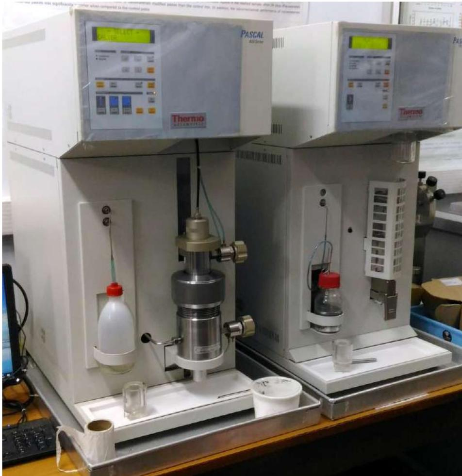
Figure 3.28 Thermo Scientific Pascal 140/440 series Mercury Intrusion Porosimetry instrument that was used in this study
