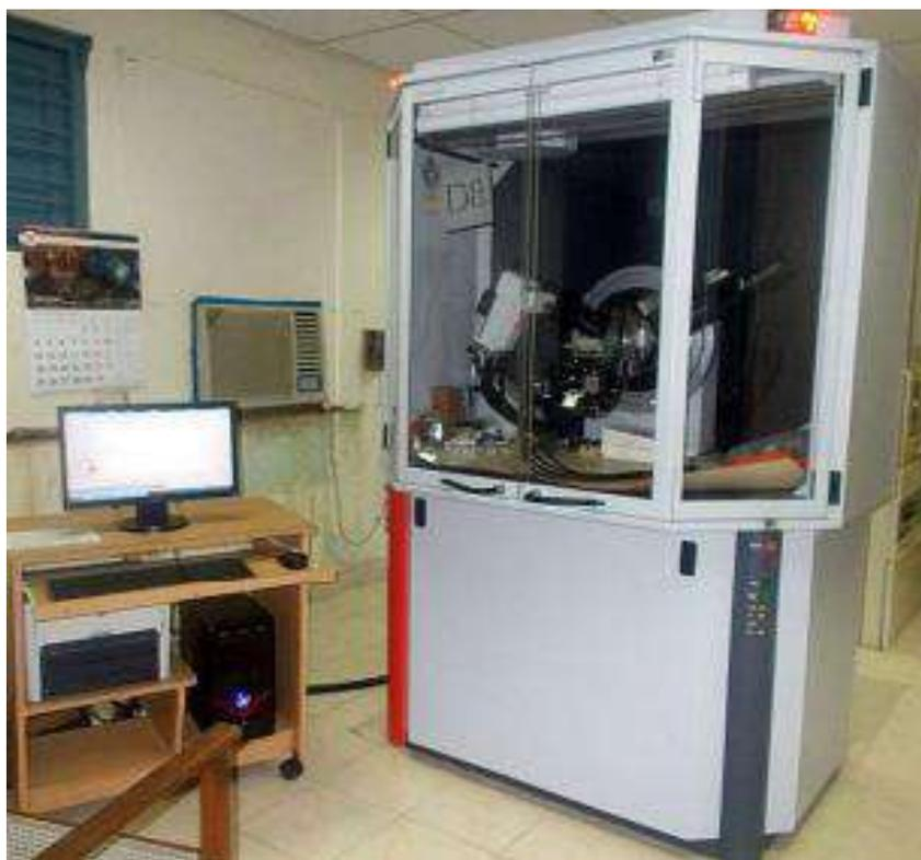
Figure 3.30 Bruker D8 Model X-ray diffraction instrument that was used in this study
