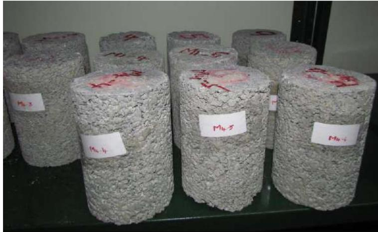
Figure 6.11 Porous concrete specimens of size 100 × 150 mm ( $\phi \times H$ ) after sectioning using diamond-tipped saw
