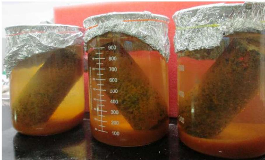
Figure 6.24 Selective chemical attack of the porous concrete specimen by storage in 0.5 M HNO<sub>3</sub> solution
