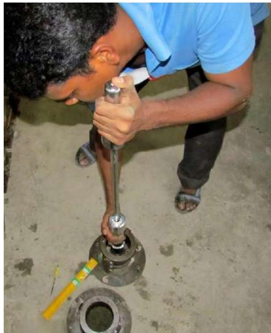
Figure 6.4 Consolidation was done using Marshall hammer having foot diameter, drop weight and free fall of 98.4 mm, 4.54 kg and 457 mm respectively
