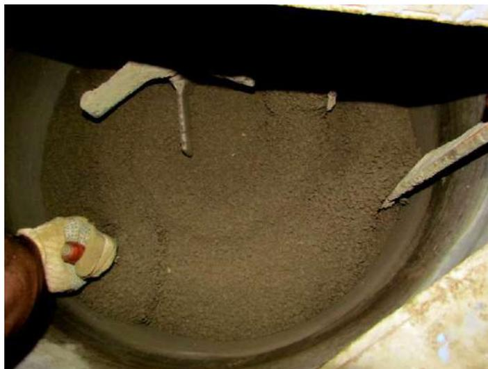
Figure 6.2 Dry blending the 53 grade Portland cement and aggregate in a laboratory concrete mixer
