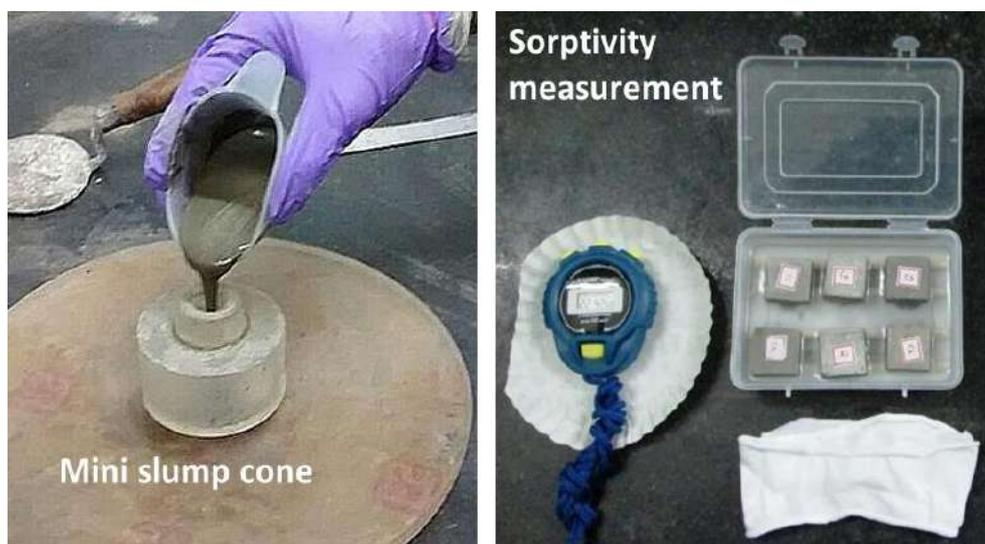
Figure 4.2 Mini slump spread (left image) and Water sorptivity test (right image)
