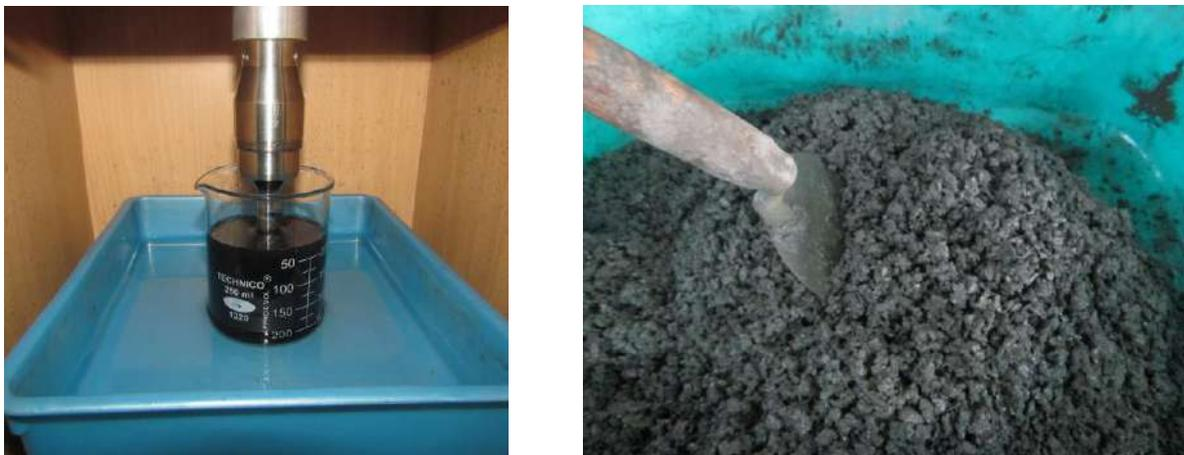
Figure 8.3 Sonication was done to the solution containing graphene using Sonics VCX-750 Vibra Cell Ultra Sonic Processor model probe sonicator (left image) and freshly prepared graphene modified porous concrete mixture (right image)
