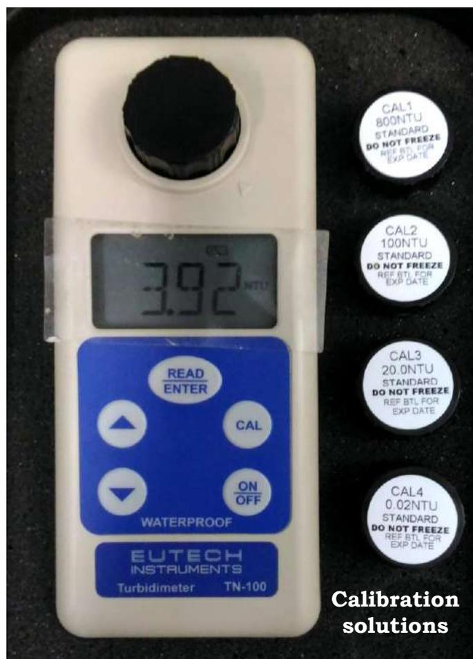
Figure 3.10 Eutech TN100 IR Turbidimeter and the standard calibration solutions having turbidity of 800 NTU, 100 NTU, 20 NTU and 0.02 NTU that were used in this study
