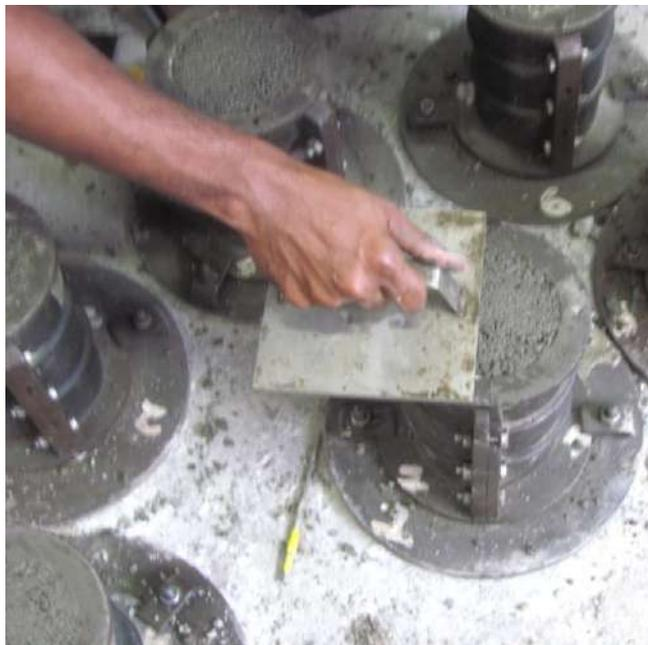
Figure 6.6 Top concrete layer was levelled and finished using a hand-held metal float
