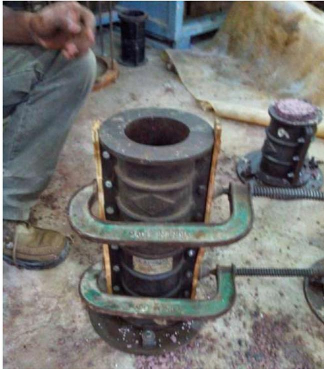
Figure 6.5 A collar arrangement was fixed to consolidate the top concrete layer that was poured inside the cylindrical iron mould
