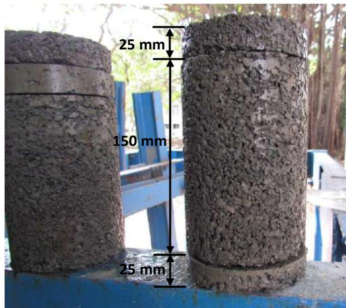
Figure 6.10 Non-permeable top and bottom concrete edges of about 25 mm thick in the specimen were removed using diamond-tipped saw
