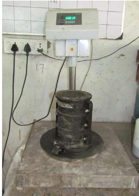
Figure 6.7 Mass of fresh and hardened porous concrete including mould was measured using a weigh balance of 0.01 g accuracy for density calculation
