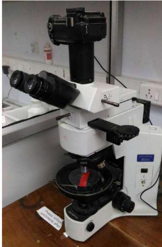
Figure 3.17 Olympus BX41 optical petrographic microscope that was used in this study
