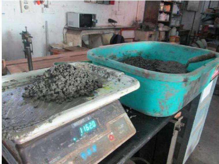
Figure 6.3 Each layer in the concrete specimen was filled by weighing the fresh concrete and then poured inside the cylindrical iron mould
