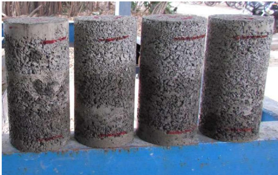
Figure 6.8 Porous concrete specimens of size  $100 \times 200$  mm ( $\phi \times H$ ) demolded after 24 hours from the mixing time of ingredients
