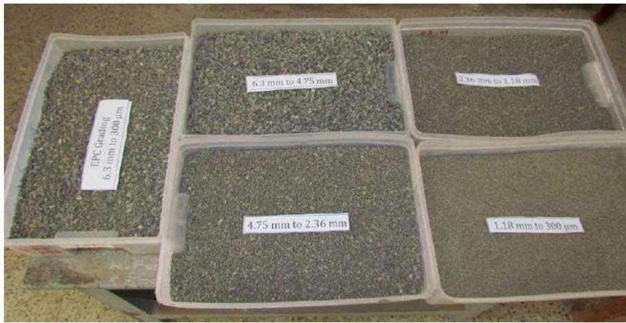
Figure 6.1 Aggregates of different sizes were separated using standard set of sieves conforming to IS 460-1 (1985)
