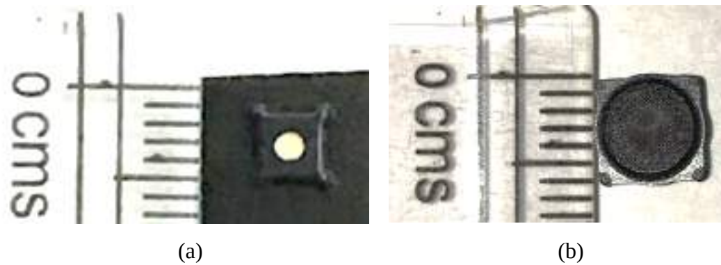
Figure C.1 (a) SHT21 sensor with the cover and (b) filter cap
