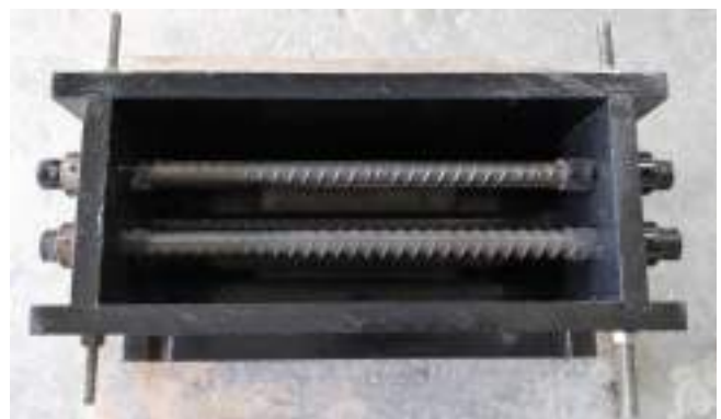
(f) Mould with steel rebars ready for casting
