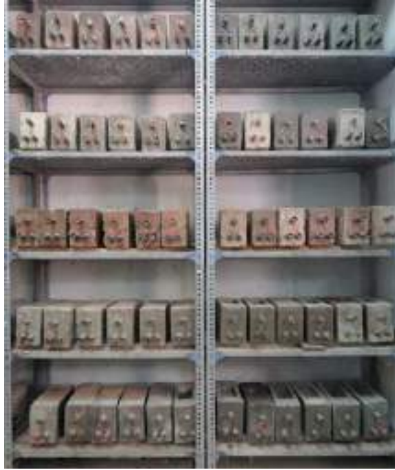
Figure 4.1 ASTM G109 specimens being exposed
