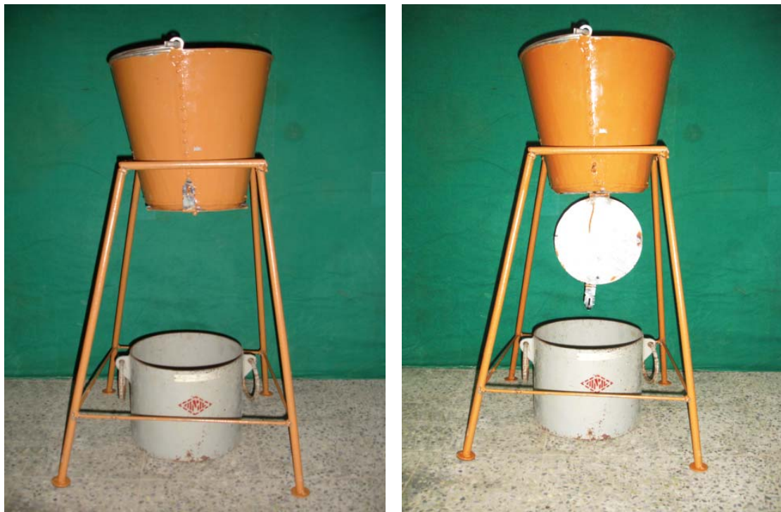
Fig. 5.1 Test set up for determining the packing density of aggregates
