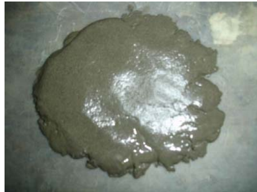
Fig. 4.2 (b) Thick cementitious paste at saturation point
