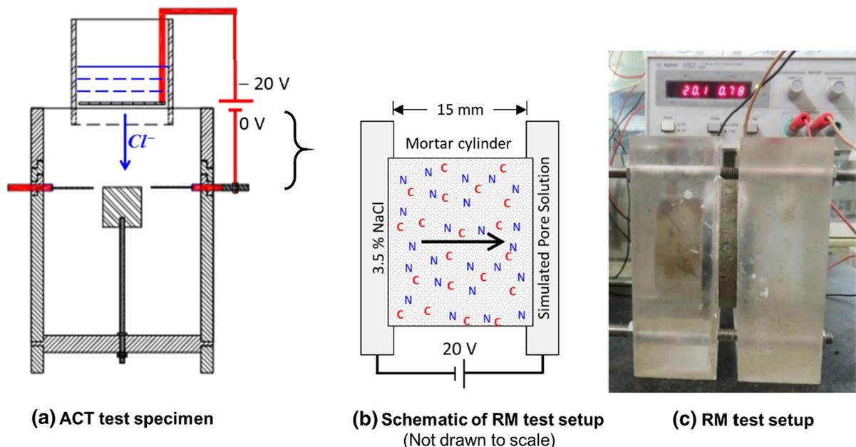
Fig. 2 Comparison of ACT specimens with RMT test
