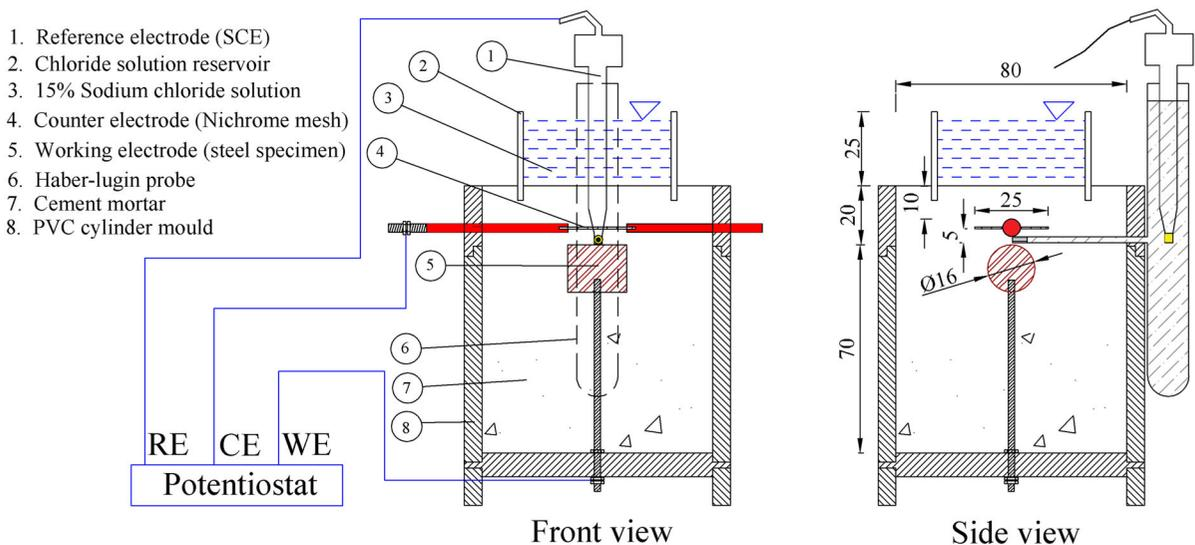
**Fig. 3** Modified accelerated chloride threshold (mACT) test layout
