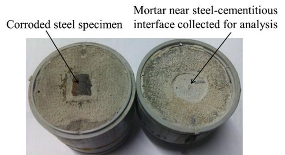
**Fig. 6** Specimen autopsied across the steel mortar interface
