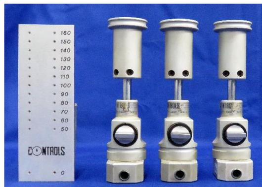
Figure 3.4(a) Axial displacement transducers
