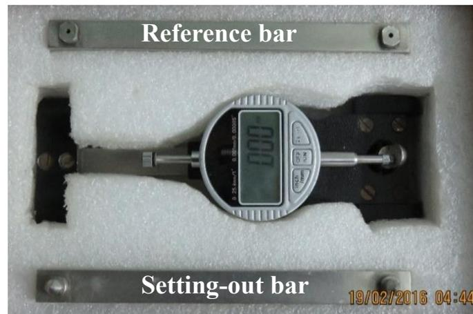
Figure 3.5 DEMEC strain gauge used for the work
