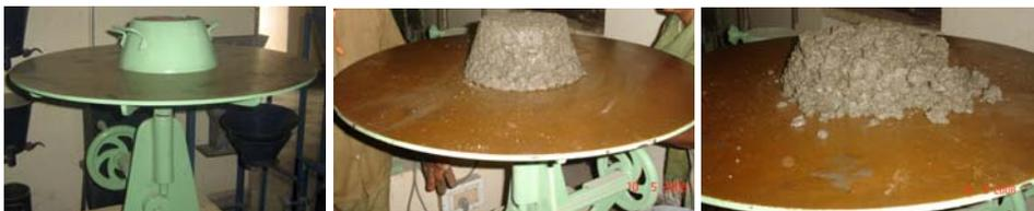
(b) Flow table test on concrete
