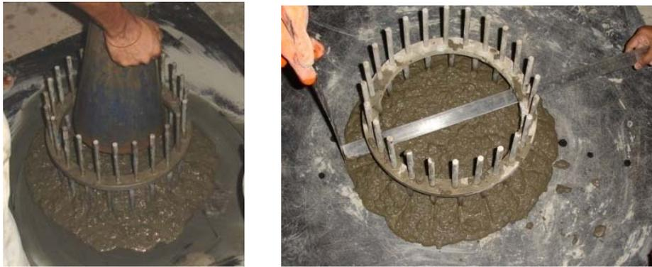
Fig. 7.16 (a) J-Ring measurement (b) J-Ring test
