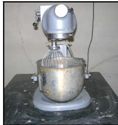
Fig. 3.11 (a) Hobart mixer with B-flat beater (b) Hobart mixer with D-wire whip
