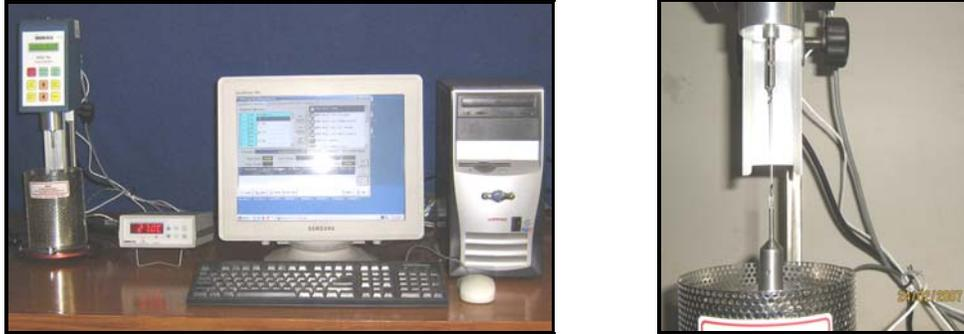
Fig. 3.6 Brookfield HA DV II +Pro viscometer (Asphalt Laboratory, IITM)
