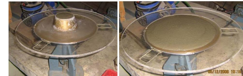
Fig. 4.3 Flow table test for mortar
