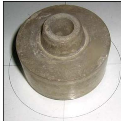
Fig. 3.4 Mini-slump cone
