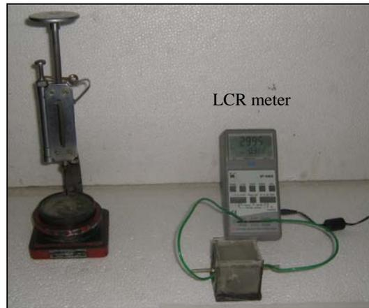
Fig. 4.20 Comparative study on setting behaviour of paste with Vicat apparatus and LCR meter
