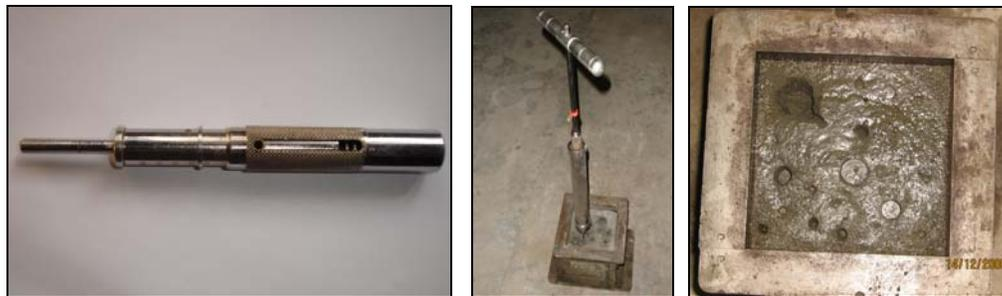
Fig.4.18 Penetration test on concrete; (a) Pocket penetrometer, (b) Penetration test on specimen (c) Impressions made on the surface during measurements
