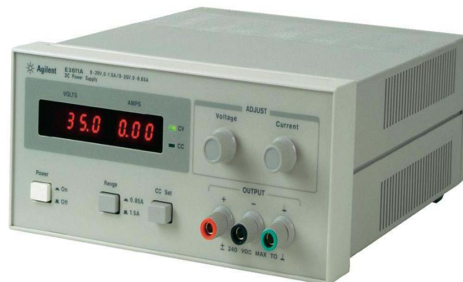
Figure 3.5 DC power supply unit used for constant power supply to the thermal probe
