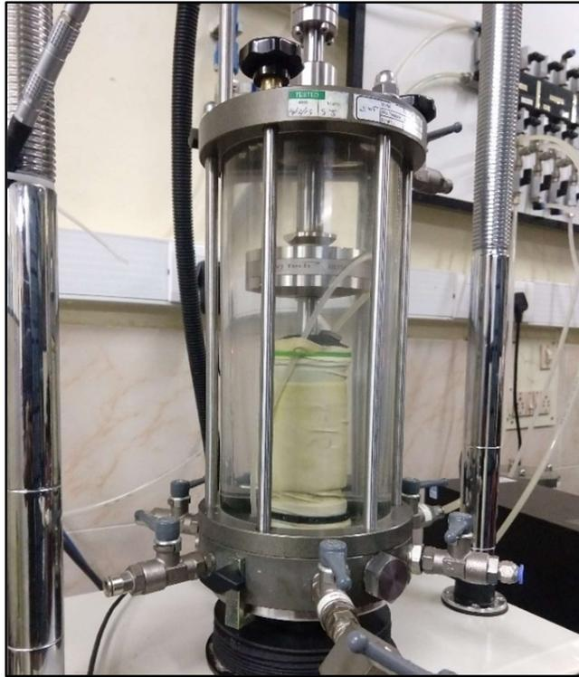
**Fig. 6.5 Photograph of the Cyclic Triaxial Test Setup**
