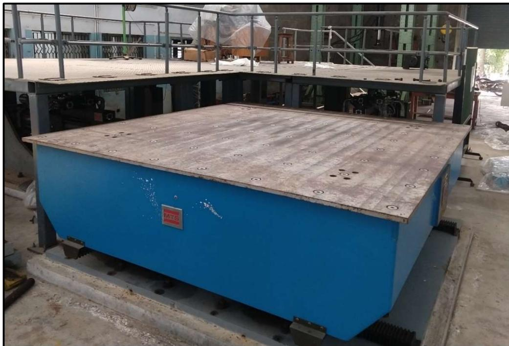
**Fig. 6.15 The biaxial shaking table at IIT Madras**
