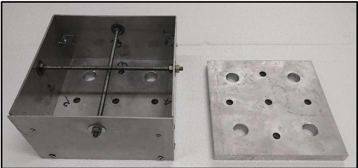
**Fig. 6.11** Photographs showing the raft (left) and the pile cap (right)
