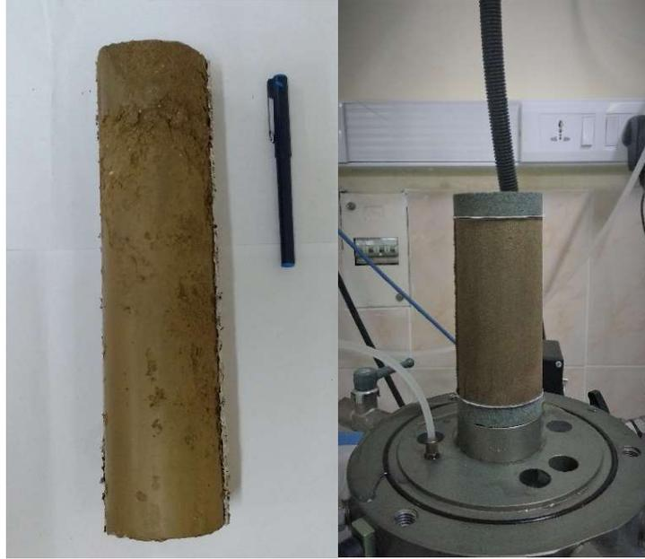
**Fig. 7.8** Photographs of (a) intact sample from 10m depth and (b) the sample trimmed to size
