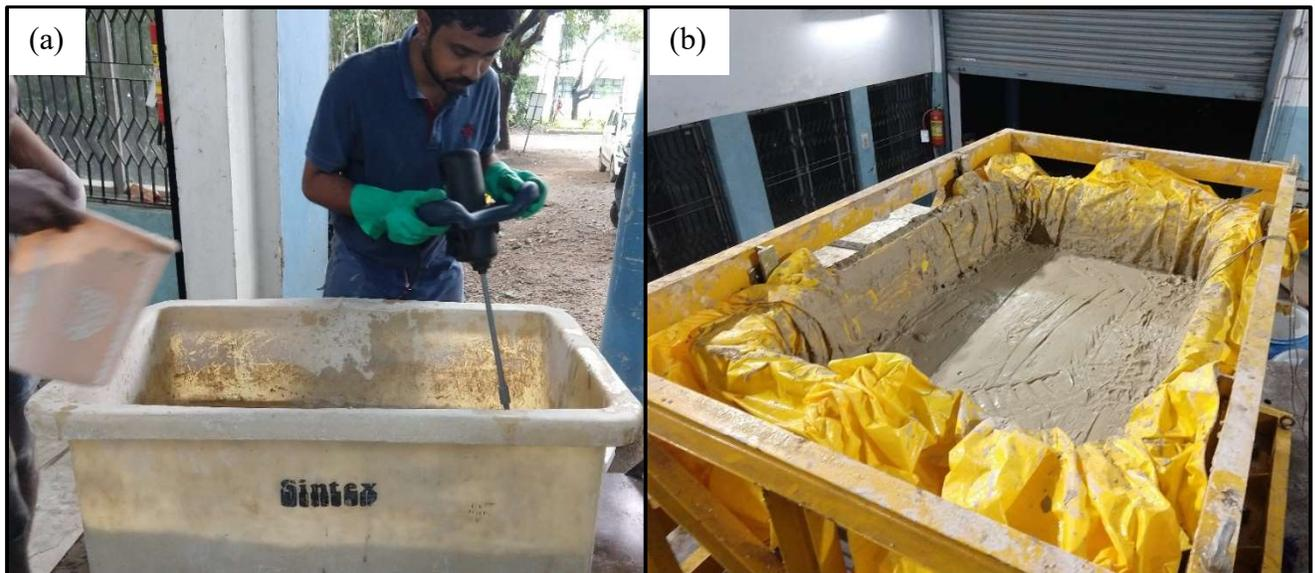
**Fig. 6.19 (a) Wet mixing using power mixer, and (b) finished clay bed**
