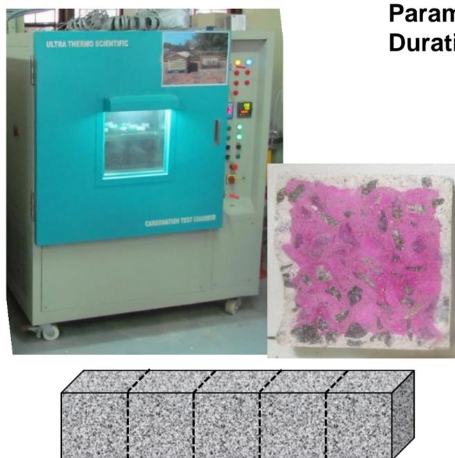
**Test: Accelerated carbonation**
