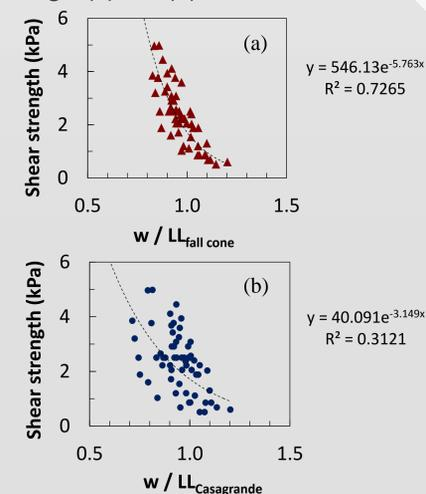
Figure 4. Shear strength versus water content ratio using (a) Fall Cone and (b) Casagrande's liquid limit
