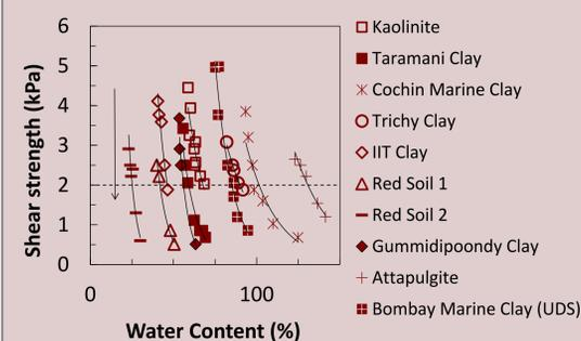
Figure 2. Variation of shear strength with water content
