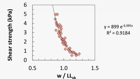
Figure 5. Shear strength versus water content ratio using strength based liquid limit
