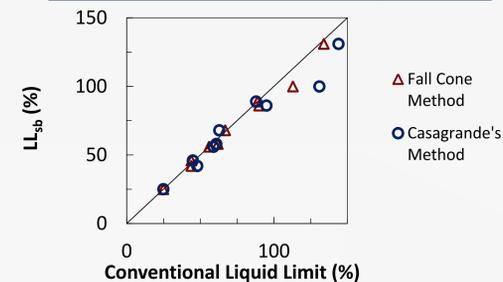
Figure 3. Comparison of strength based liquid limit and Casagrande's and fall cone liquid limit values
