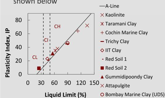
Figure 1. Position of soils in the Plasticity Chart as per Indian Standard Soil Classification System
