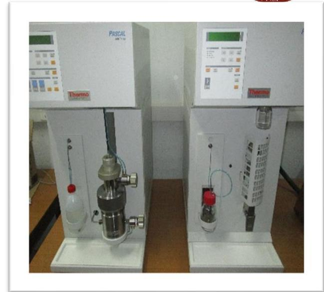
Mercury intrusion porosimeter
