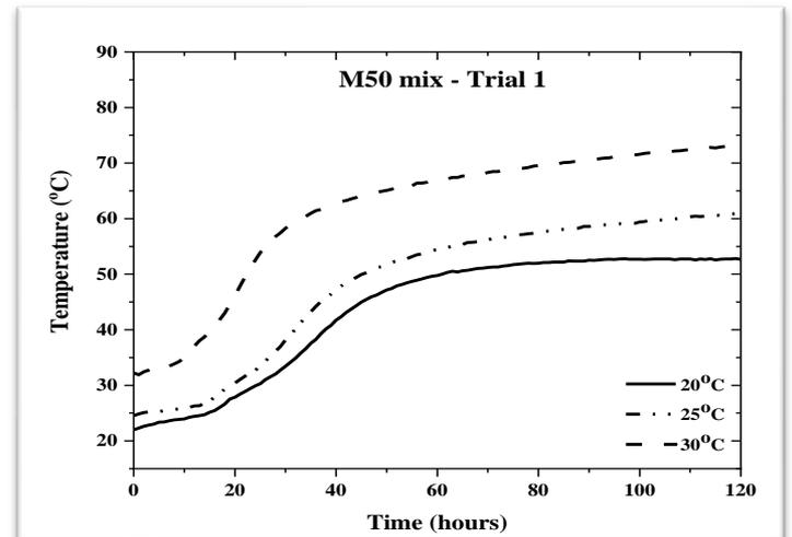
Temperature profile of concrete placed at different temperatures
