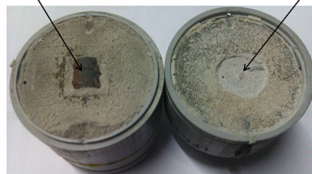
Fig. 6 Specimen autopsied across the steel mortar interface
