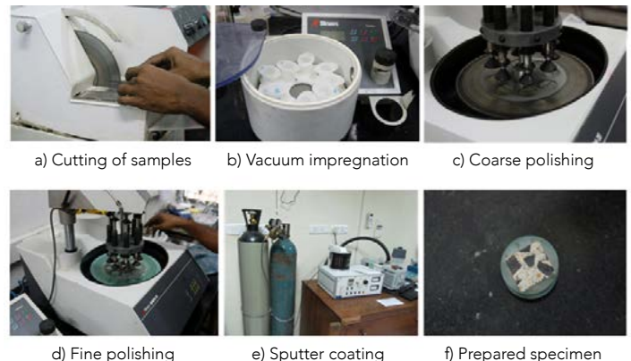
Figure 5: Sample preparation for SEM - BSE Imaging.
