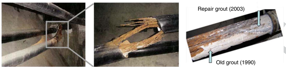
FIGURE 3. Failure of a tendon in a bridge within 4 y after repair (Courtesy: Hansen 28 ).
