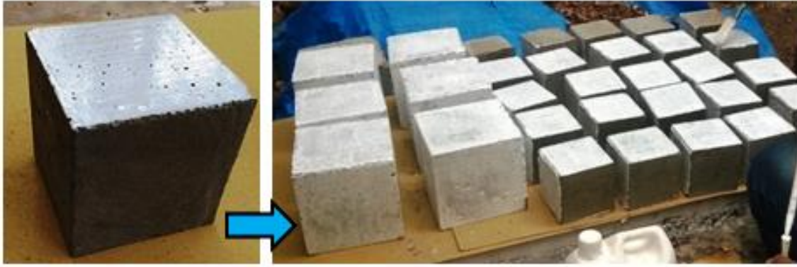
Figure 1. Application of curing compound on the cube specimens
