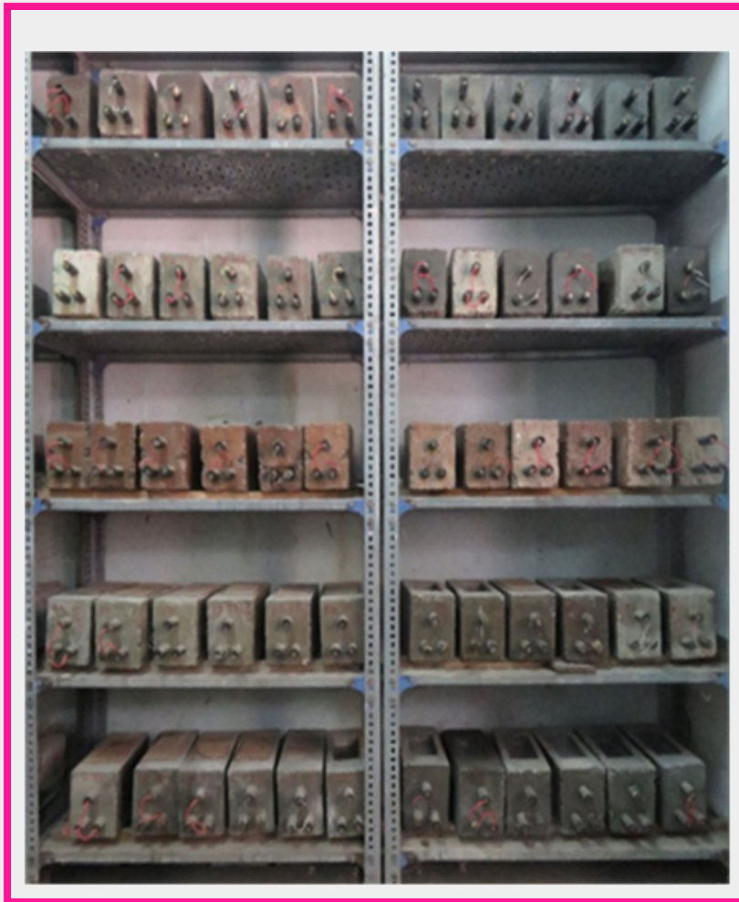
Figure 1. ASTM G109 specimens being exposed. +
