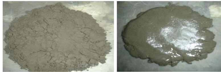
Apparatus for Puntke test (top), mix before saturation limit (bottom left), mix after reaching saturation limit (bottom right)
