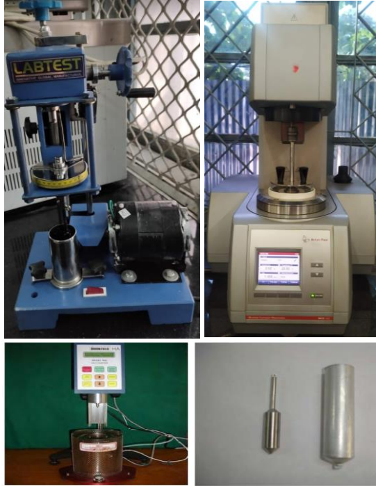
Vane shear apparatus (top left), Rheometer (top right), Brookfield viscometer with spindle (bottom)
